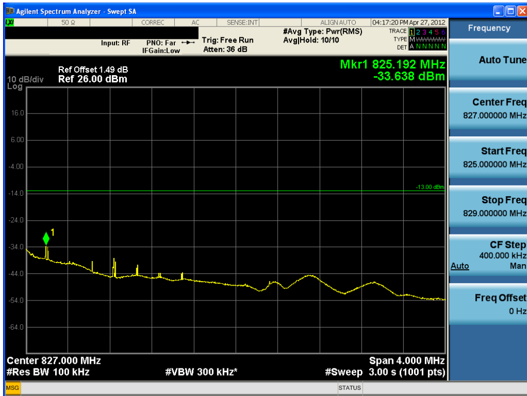
Plot 7-10. 4MHz Span Plot (BC10 CDMA Ch. 684)
