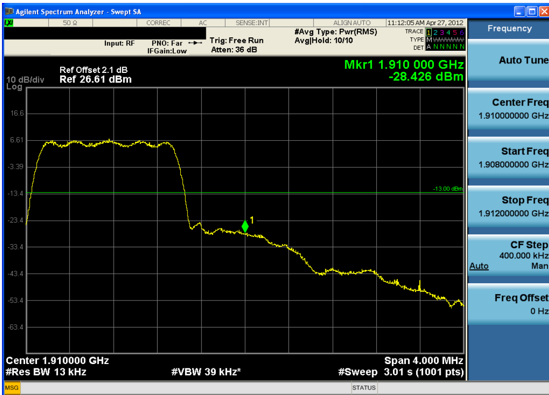
Plot 7-22. Band Edge Plot (PCS CDMA Mode – Ch. 1175)
