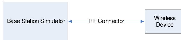
Figure 12-1 Power Measurement Setup
