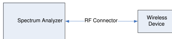
Figure 14-1 Power Measurement Setup
