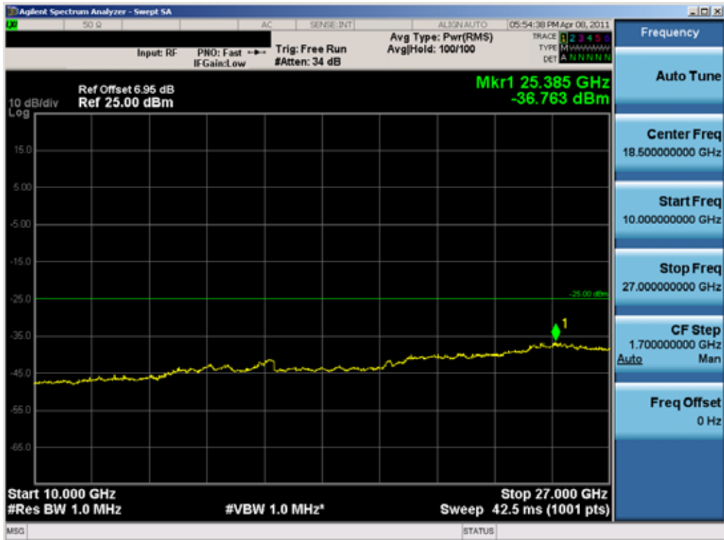
Plot 8-12. Conducted Spurious Plot (WiMAX – High Channel)
