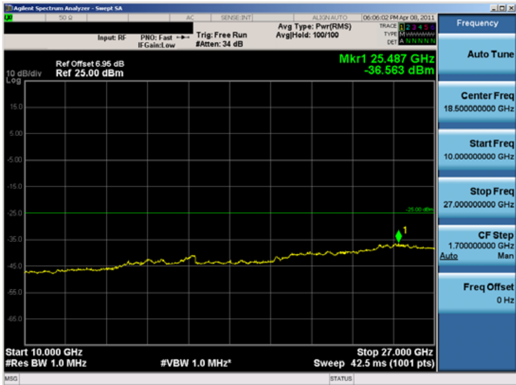
Plot 7-12. Conducted Spurious Plot (WiMAX – High Channel)
