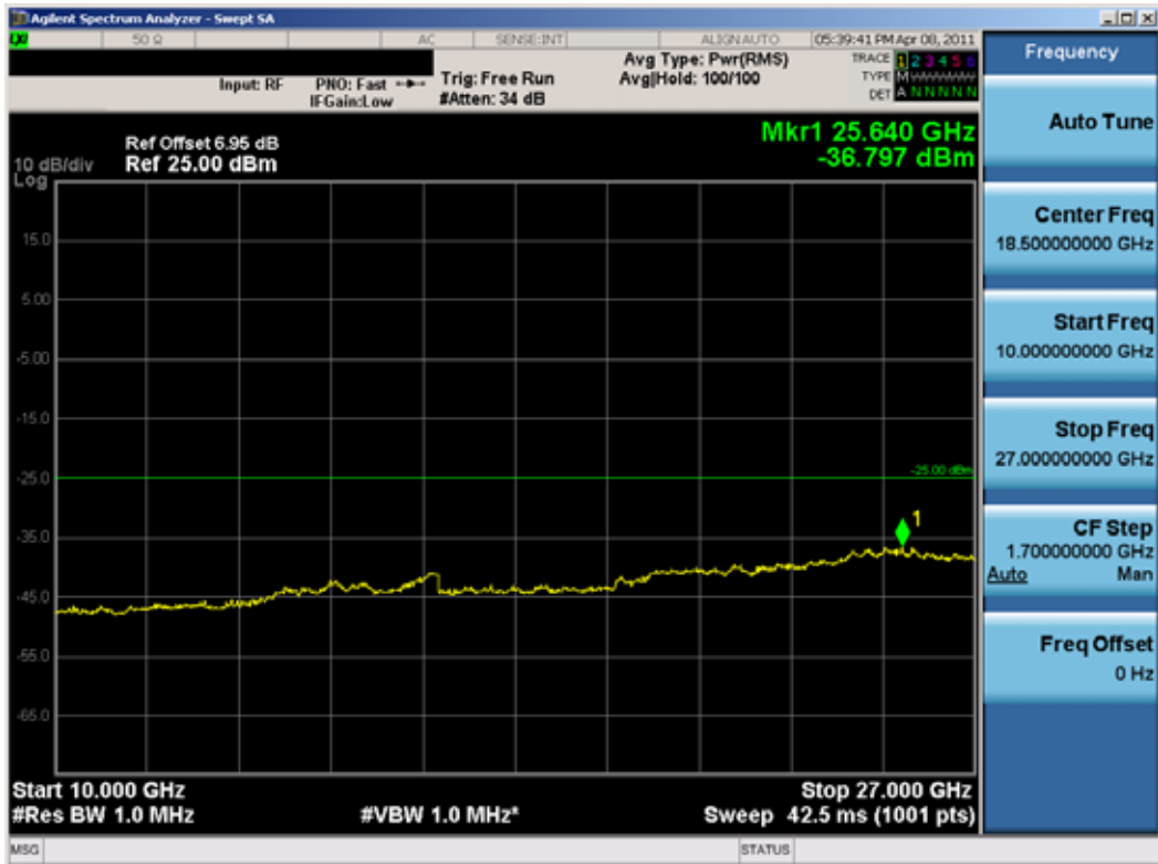
Plot 8-6. Conducted Spurious Plot (WiMAX – Mid Channel)
