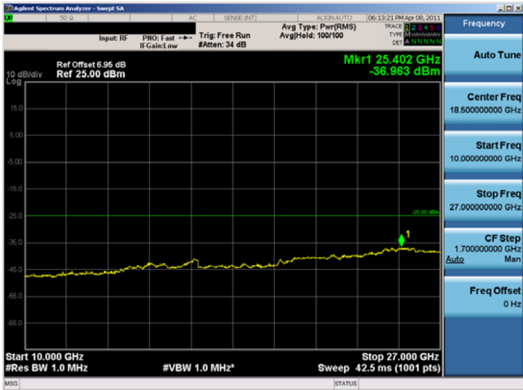
Plot 7-6. Conducted Spurious Plot (WiMAX – Mid Channel)
