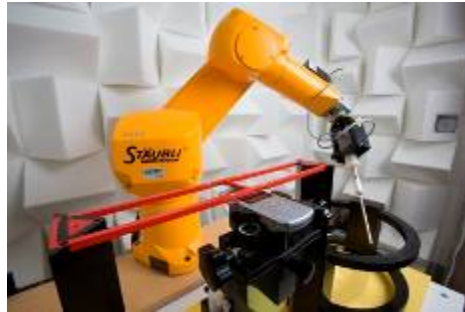
Figure 5-5 SPEAG Robotic System
