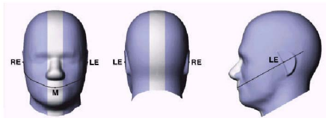
Figure 9-2 Front, back and side view of SAM Twin Phantom
