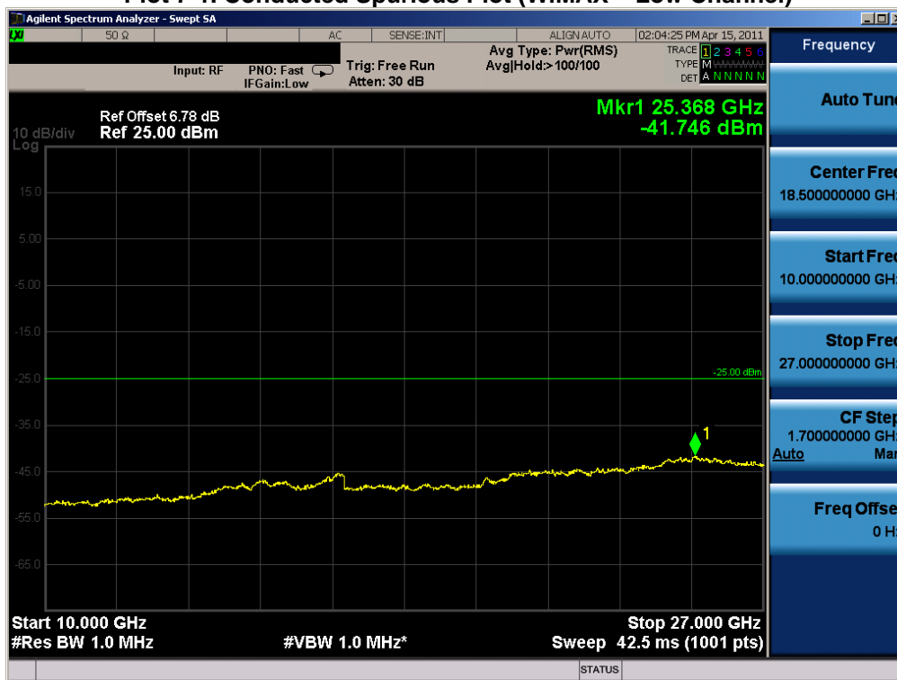
Plot 7-2. Conducted Spurious Plot (WiMAX – Low Channel)
