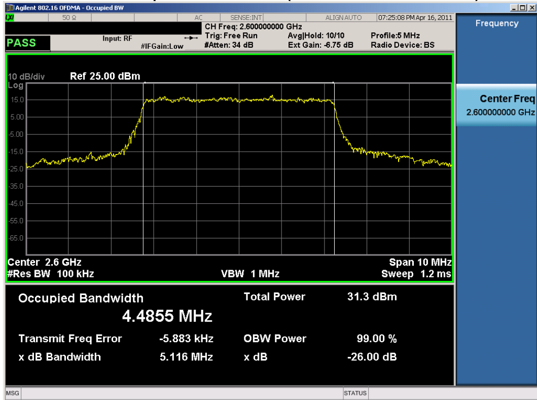
Plot 7-8. Occupied Bandwidth Plot (WiMAX 16-QAM – Mid Channel)
