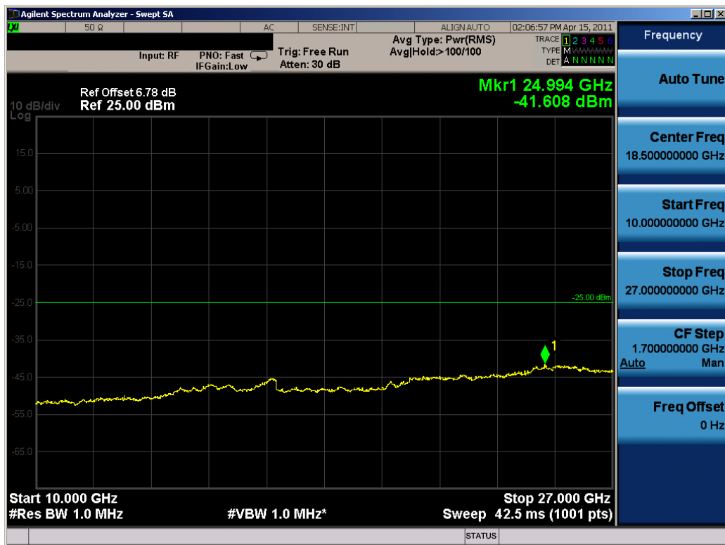
Plot 7-12. Conducted Spurious Plot (WiMAX – High Channel)
