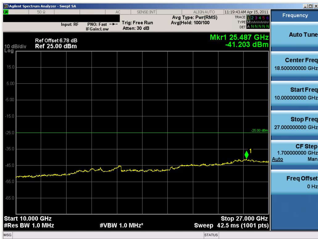
Plot 8-12. Conducted Spurious Plot (WiMAX – High Channel)
