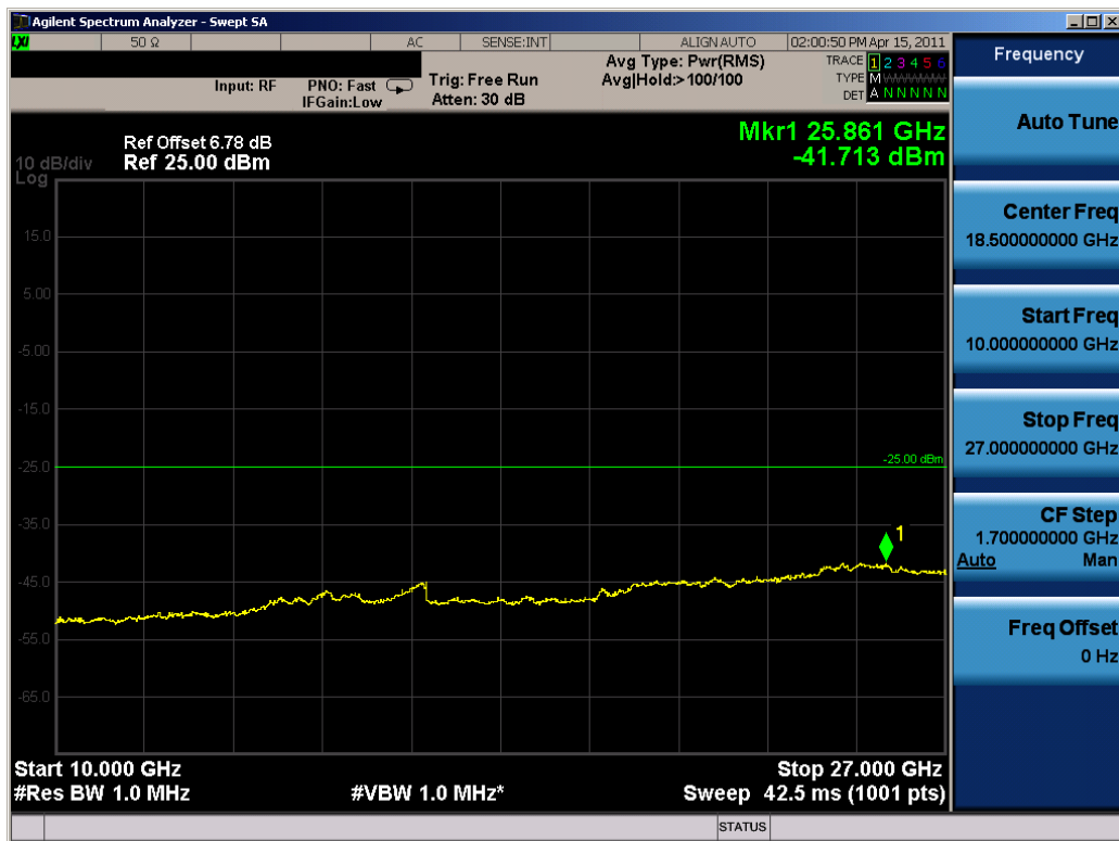
Plot 7-6. Conducted Spurious Plot (WiMAX – Mid Channel)
