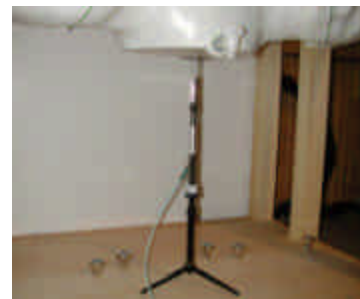
Figure 12.1 Dipole Validation Test Setup
