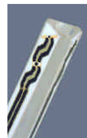
Figure 3.2 Probe Thick-Film Technique
