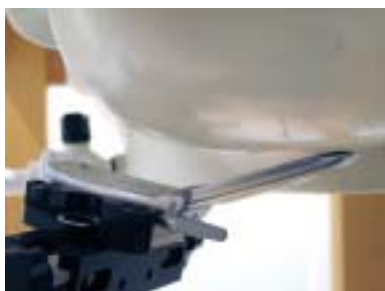
Figure 8.13 Left Head SAR Test Setup -- Ear/Tilt 15° Position--
