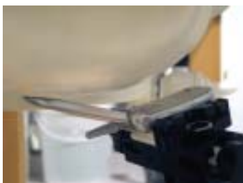
Figure 8.7 Right Head SAR Test Setup -- Ear / Tilt 15° Position --
