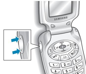
In Standby mode, you can adjust the key beep volume using these keys.
