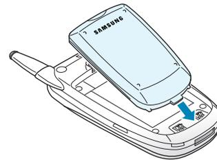
2. Press the battery down until it snaps into place.
