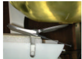
Figure 14.9 Left Head SAR Test Setup -- Ear / Tilt Position --
