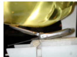
Figure 14.10 Right Head SAR Test Setup -- Ear / 15° Tilt Position --
