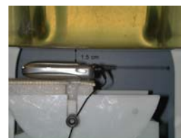
Figure 14.11 Body SAR Test Setup -- w/o Holster --
