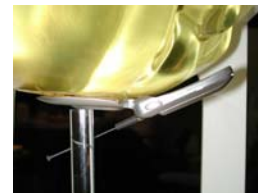
Figure 14.6 Right Head SAR Test Setup -- Cheek / Touch Position --
