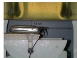
Figure 14.13 Body SAR Test Setup -- w/o Holster --
