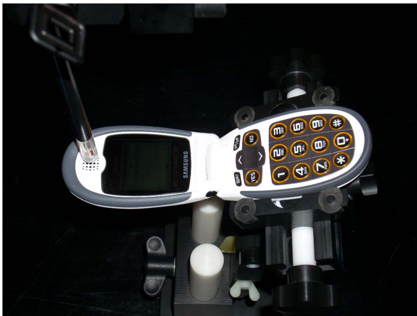
Figure 13-1 Test Setup for Wireless Device
