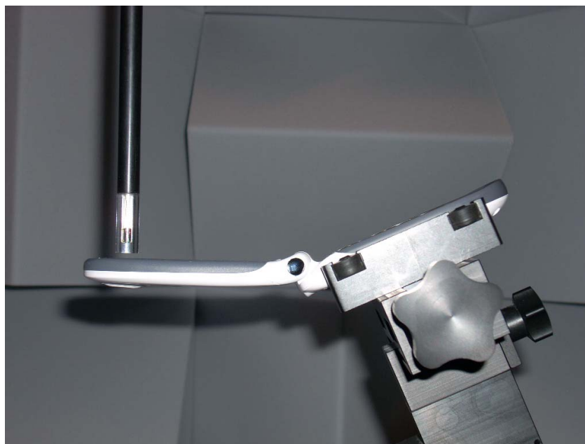
Figure 13-2 Test Setup for Wireless Device
