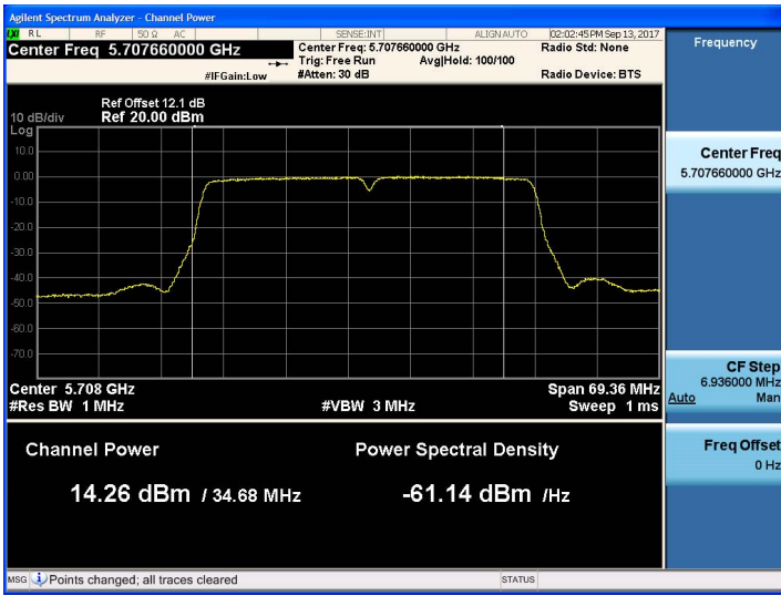
802.11ac_VHT40 UNII 2C Band Average Power CH.142
