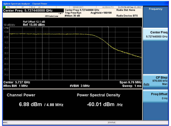
802.11ac_VHT20 UNII 3 Band Average Power CH.144
