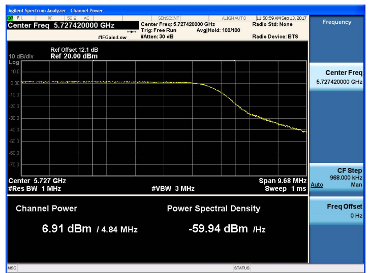
802.11n_HT20 UNII 3 Band Average Power CH.144
