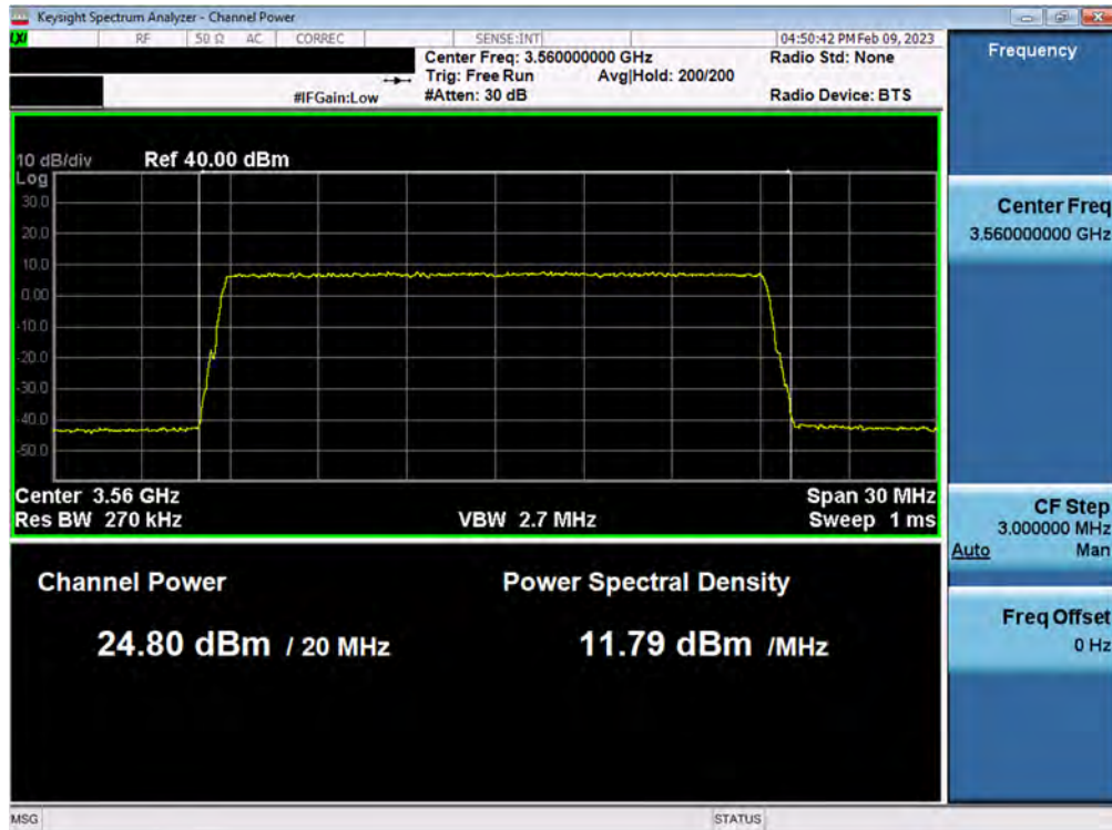
Plot 37. Conducted PSD, 3.56GHz, 20MHz BW – ANT5, SAS Granted maxEIRP 29dBm/MHz (NR)
