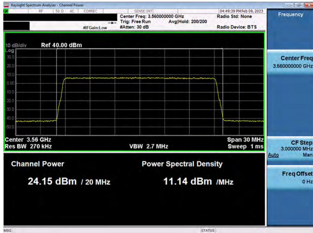
Plot 36. Conducted PSD, 3.56GHz, 20MHz BW – ANT4, SAS Granted maxEIRP 29dBm/MHz (NR)
