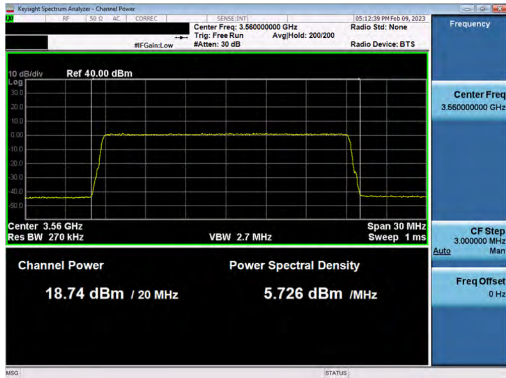
Plot 41. Conducted PSD, 3.56GHz, 20MHz BW – ANT1, SAS Granted maxEIRP 23dBm/MHz (NR)
