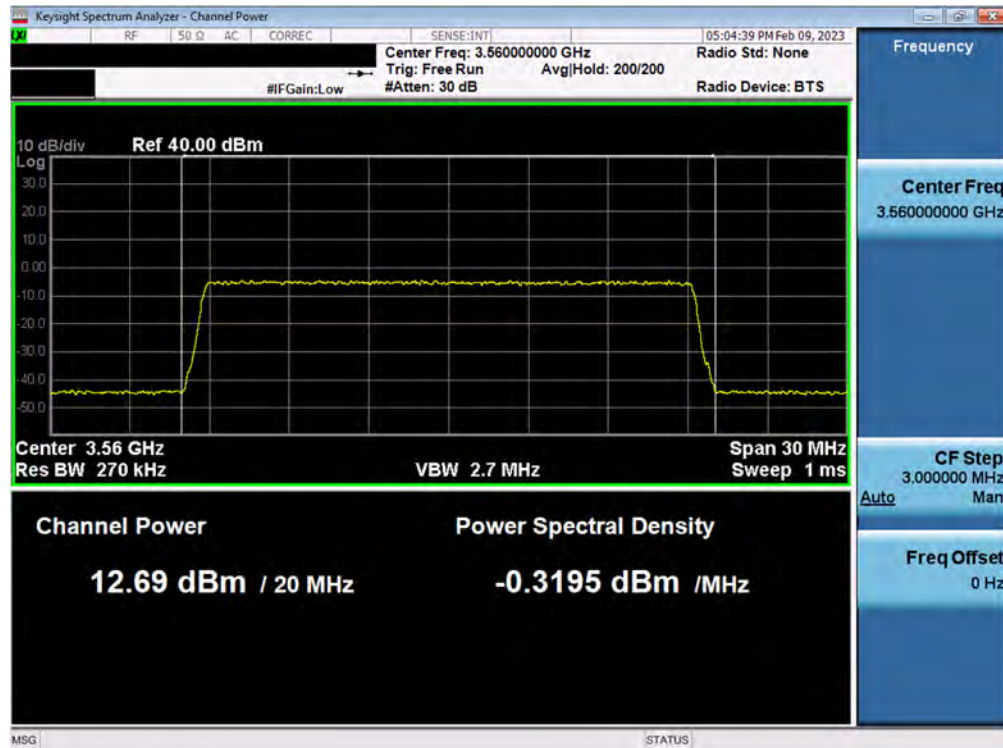
Plot 54. Conducted PSD, 3.56GHz, 20MHz BW – ANT6, SAS Granted maxEIRP 17dBm /MHz (NR)
