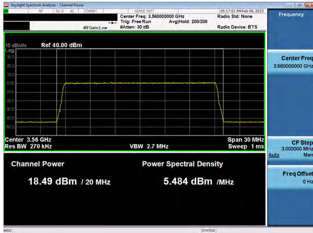
Plot 46. Conducted PSD, 3.56GHz, 20MHz BW – ANT6, SAS Granted maxEIRP 23dBm /MHz (NR)
