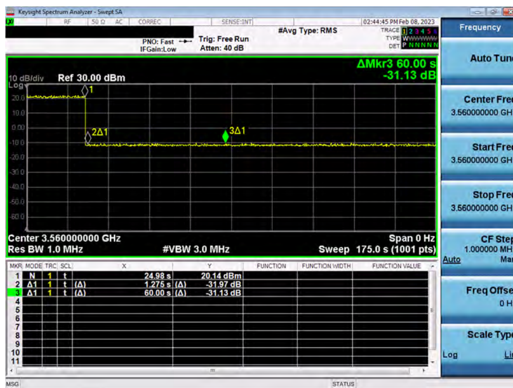
Plot 22. Conducted Measurement - RF transmission stops within 60s. The SAS message is indicated by Marker 1 (X) (WINNF.FT.C.DRG.1) – NR
