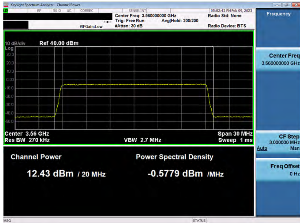
Plot 56. Conducted PSD, 3.56GHz, 20MHz BW – ANT8, SAS Granted maxEIRP 17dBm /MHz (NR)
