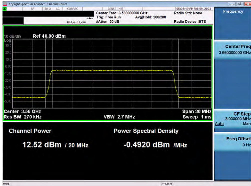
Plot 52. Conducted PSD, 3.56GHz, 20MHz BW – ANT4, SAS Granted maxEIRP 17dBm /MHz (NR)
