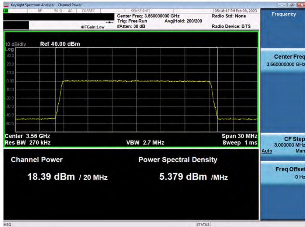
Plot 48. Conducted PSD, 3.56GHz, 20MHz BW – ANT8, SAS Granted maxEIRP 23dBm /MHz (NR)
