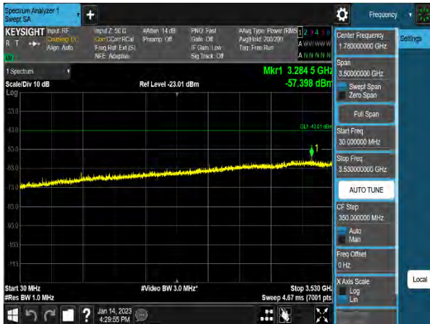
Plot 8-256. Conducted Spurious Emission Plot 30 MHz to 3.53 GHz (n48_2NC_40M+40M_QPSK - Mid Channel_2T, Port 3)
