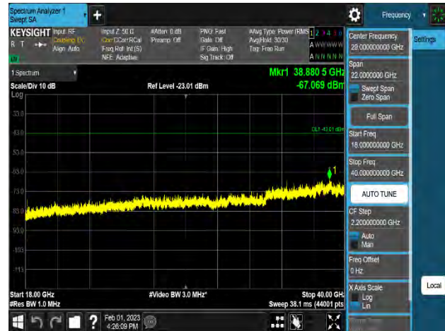
Plot 8-251. Conducted Spurious Emission Plot 18 GHz to 40 GHz (n48_1C_10M_QPSK - High Channel_2T, Port 3)
