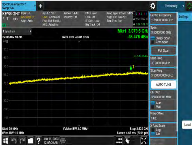
Plot 8-248. Conducted Spurious Emission Plot 30 MHz to 3.53 GHz (n48_1C_10M_QPSK - High Channel_2T, Port 3)
