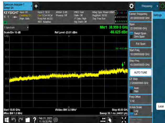
Plot 8-259. Conducted Spurious Emission Plot 18 GHz to 40 GHz (n48_2NC_40M+40M_QPSK - Mid Channel_2T, Port 3)
