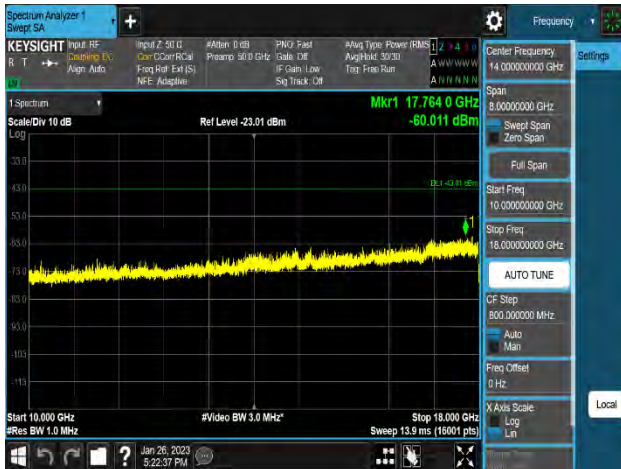
Plot 8-250. Conducted Spurious Emission Plot 10 GHz to 18 GHz (n48_1C_10M_QPSK - High Channel_2T, Port 3)
