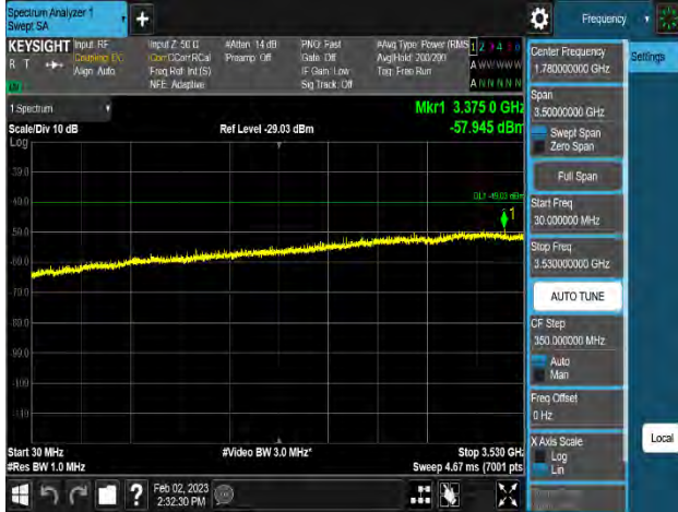
Plot 8-260. Conducted Spurious Emission Plot 30 MHz to 3.53 GHz (n48_1C_10M_QPSK - Mid Channel_8T, Port 8)
