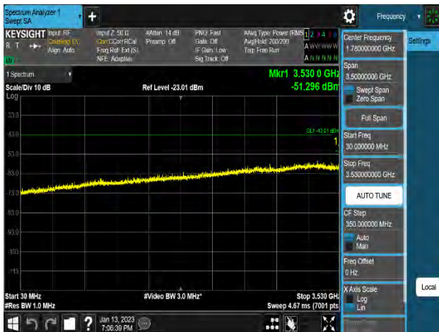
Plot 8-252. Conducted Spurious Emission Plot 30 MHz to 3.53 GHz (n48_2C_40M+40M_256QAM - Low Channel_2T, Port 4)
