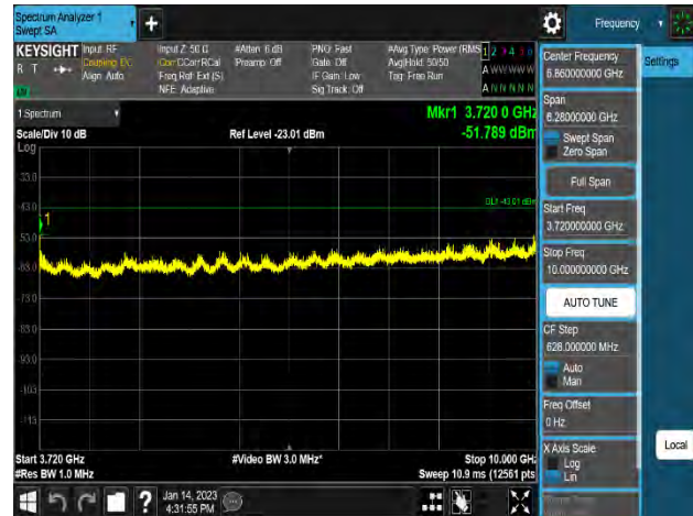
Plot 8-257. Conducted Spurious Emission Plot 3.72 GHz to 10 GHz (n48_2NC_40M+40M_QPSK - Mid Channel_2T, Port 3)
