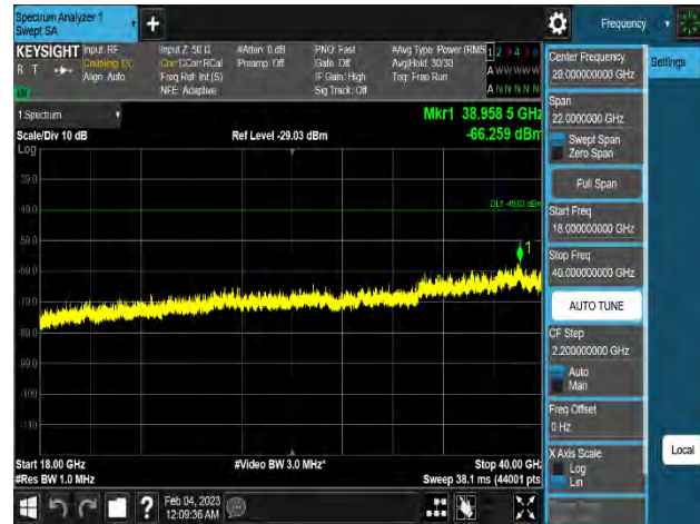
Plot 8-263. Conducted Spurious Emission Plot 18 GHz to 40 GHz (n48_1C_10M_QPSK - Mid Channel_8T, Port 8)
