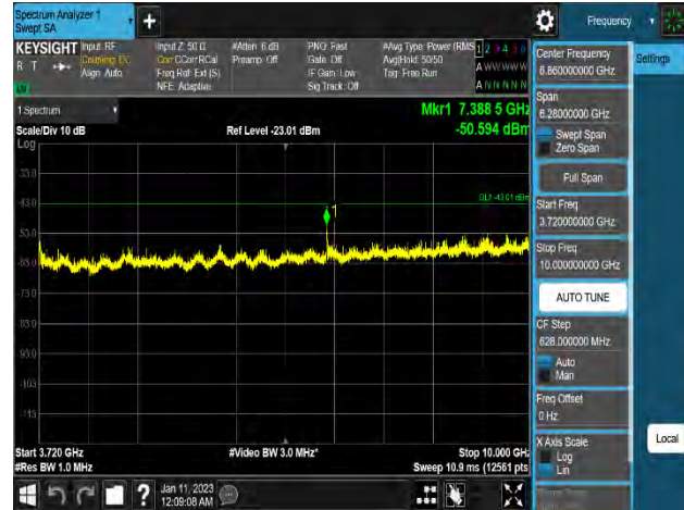
Plot 8-249. Conducted Spurious Emission Plot 3.72 GHz to 10 GHz (n48_1C_10M_QPSK - High Channel_2T, Port 3)
