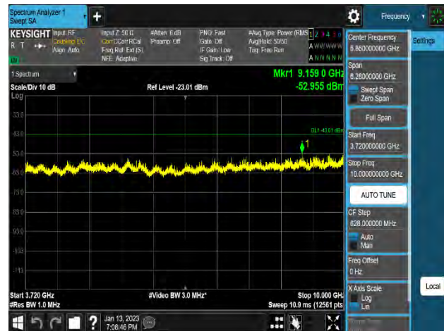
Plot 8-253. Conducted Spurious Emission Plot 3.72 GHz to 10 GHz (n48_2C_40M+40M_256QAM - Low Channel_2T, Port 4)
