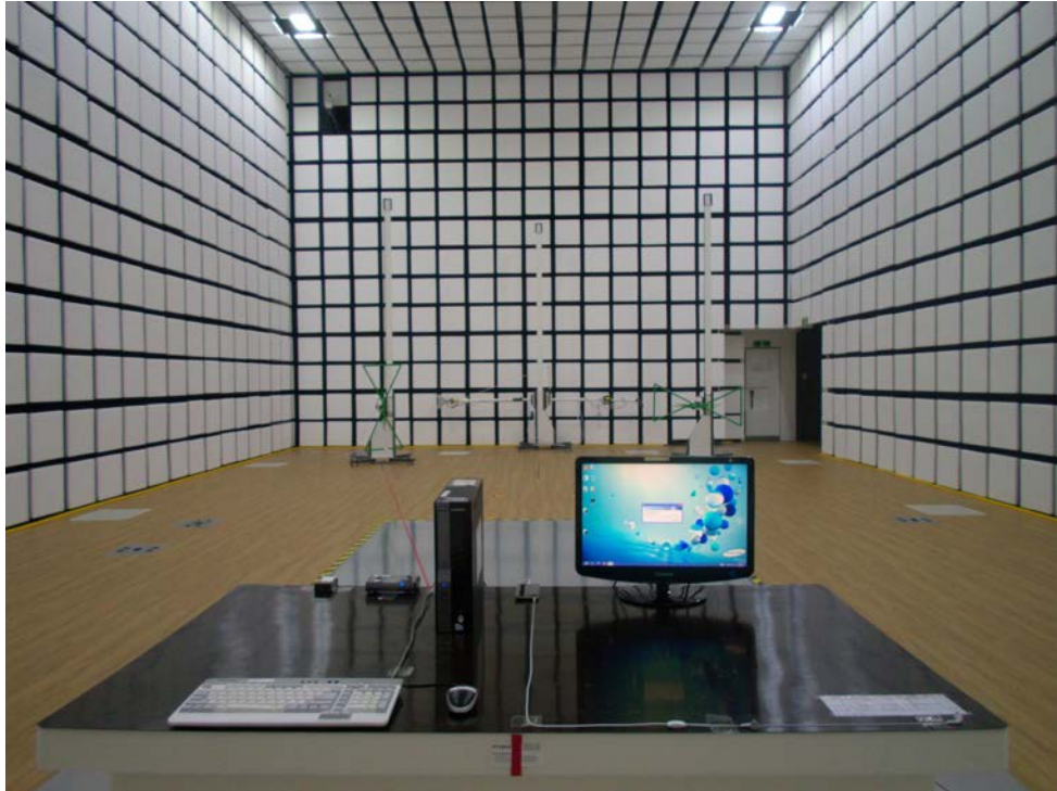
[ Radiated Disturbance for Below 1 GHz – Front ]
