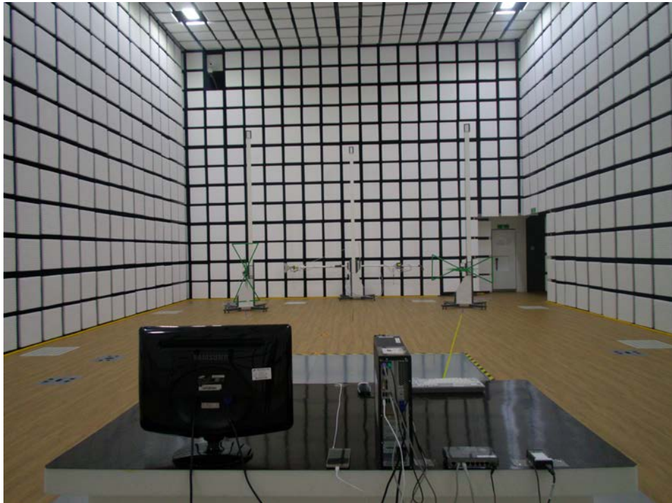
[ Radiated Disturbance for Below 1 GHz – Rear ]
