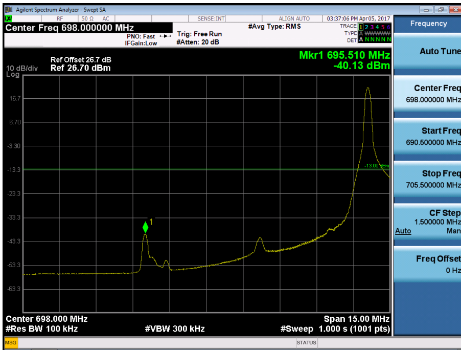
Band 17 Lower Band Edge Plot (10M BW Ch.23780 QPSK_RB1 OFFSET0)
