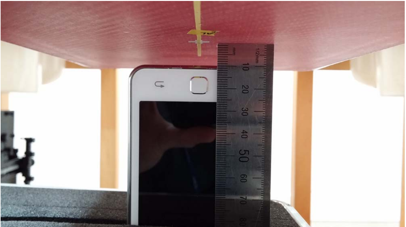
[Distance of 1.0 cm from the EUT]
