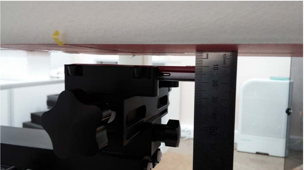
[Distance of 1.0 cm from the EUT]
