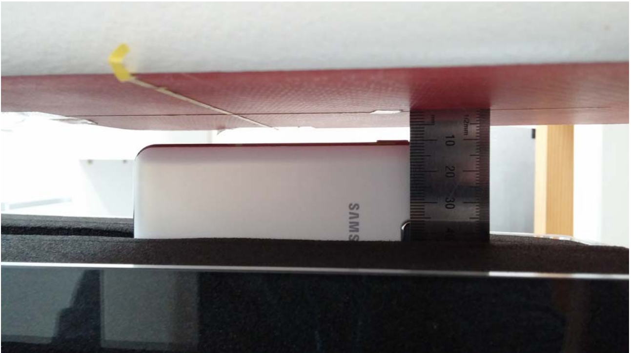
[Distance of 1.0 cm from the EUT]
