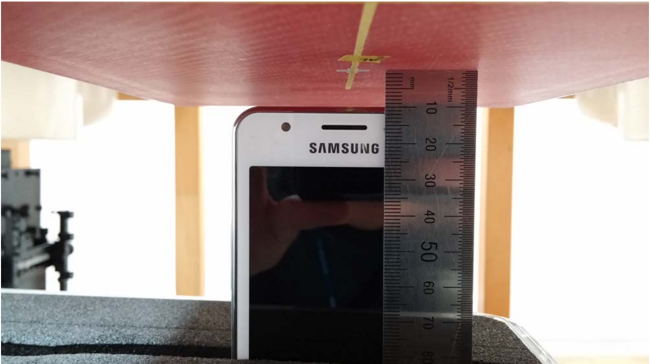
[Distance of 1.0 cm from the EUT]
