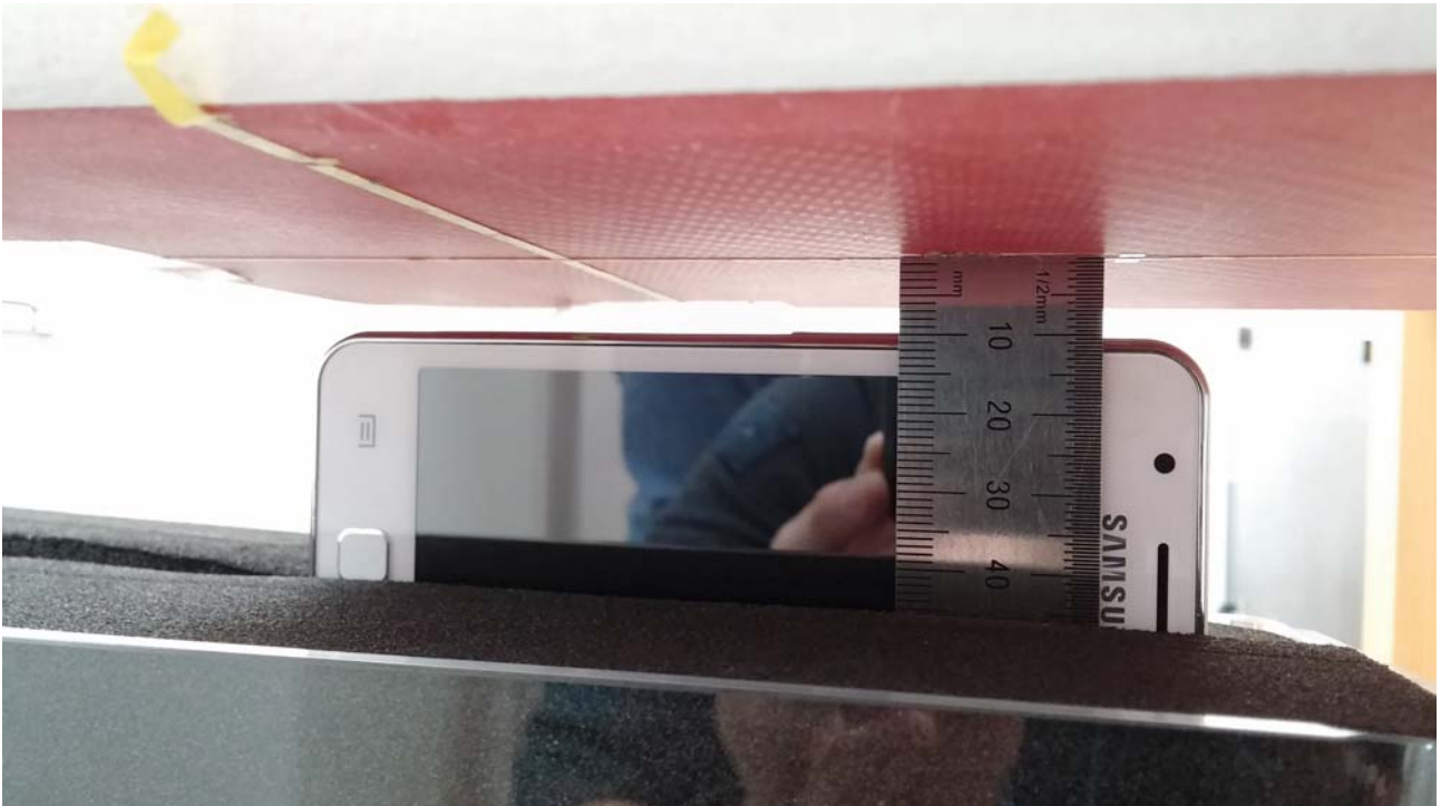
[Distance of 1.0 cm from the EUT]
