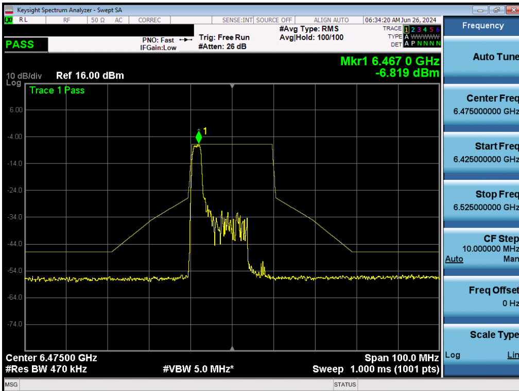
Plot 7-230. In Band Emissions Plot MIMO ANT1 (20MHz BW 802.11ax/be (26 Tones) (UNII Band 6) – Ch. 105)
