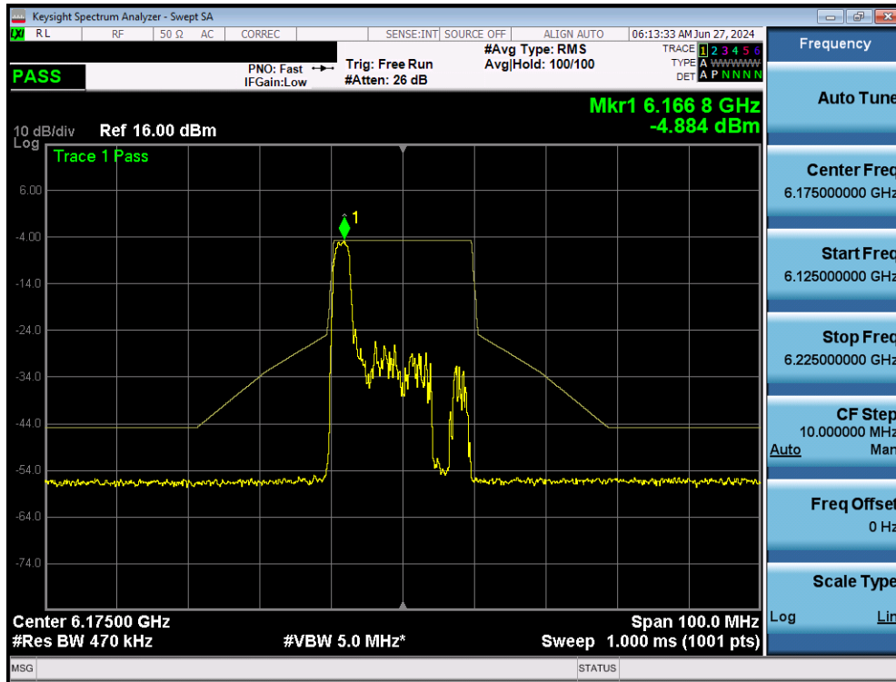
Plot 7-225. In Band Emissions Plot MIMO ANT1 (20MHz BW 802.11 ax/be (26 Tones) (UNII Band 5) – Ch. 45)
