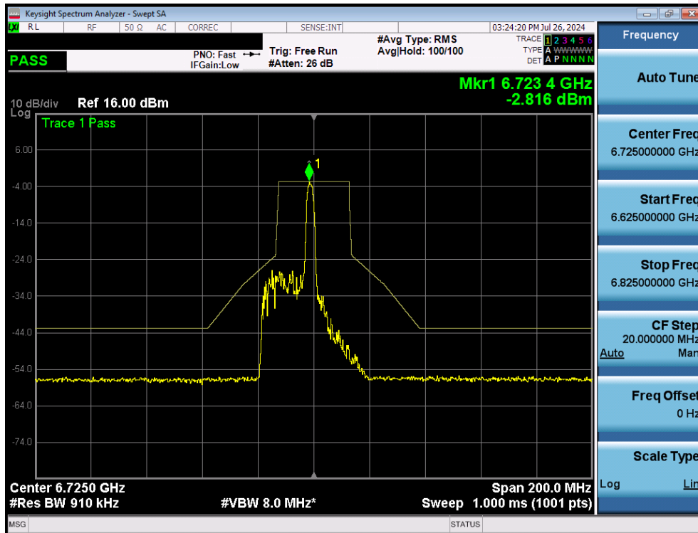
Plot 7-236. In Band Emissions Plot MIMO ANT1 (40MHz BW 802.11ax/be (26 Tones) (UNII Band 7) – Ch. 155)
