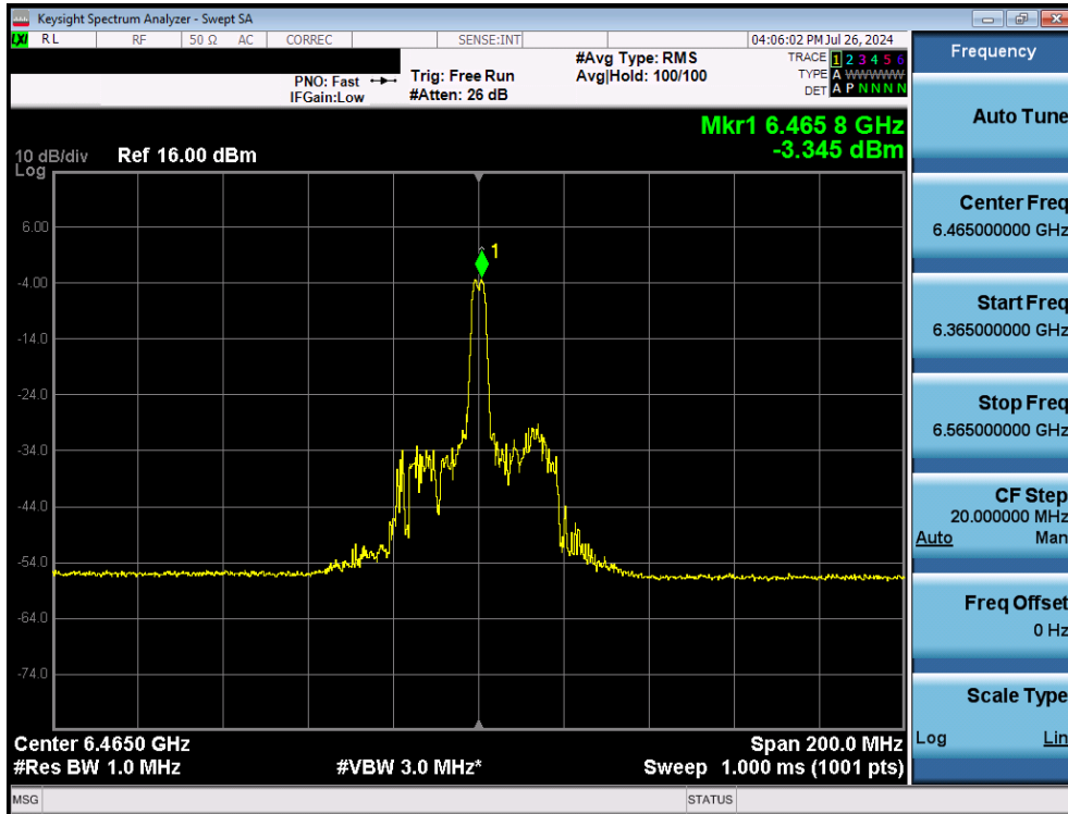
Plot 7-120. Power Spectral Density Plot MIMO ANT1 (80MHz BW 802.11ax/be (26 Tones) (UNII Band 6) – Ch. 103)
