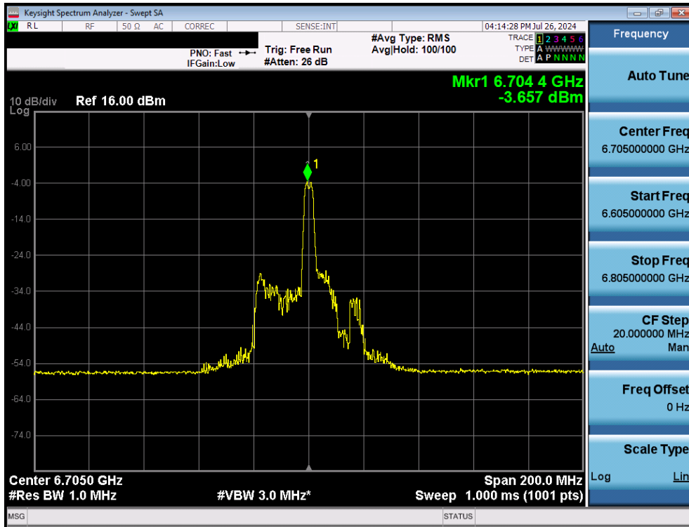
Plot 7-125. Power Spectral Density Plot MIMO ANT1 (80MHz BW 802.11ax/be (26 Tones) (UNII Band 7) – Ch. 151)
