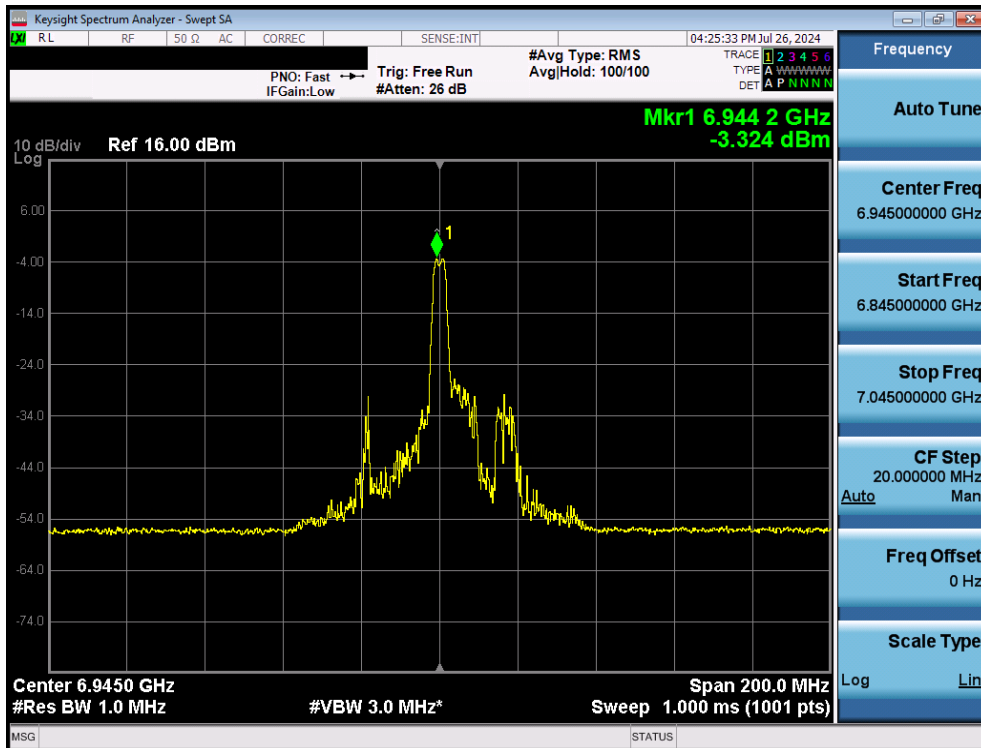
Plot 7-130. Power Spectral Density Plot MIMO ANT1 (80MHz BW 802.11ax/be (26 Tones) (UNII Band 8) – Ch. 199)
