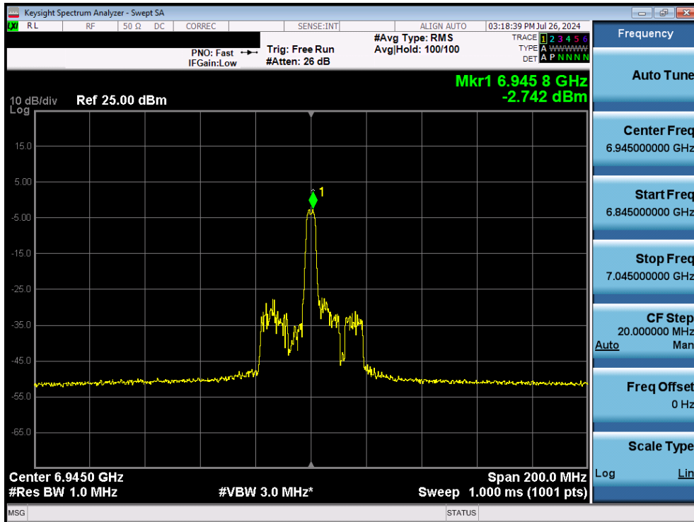
Plot 7-186. Power Spectral Density Plot MIMO ANT2 (80MHz BW 802.11ax/be (26 Tones) (UNII Band 8) – Ch. 199)
