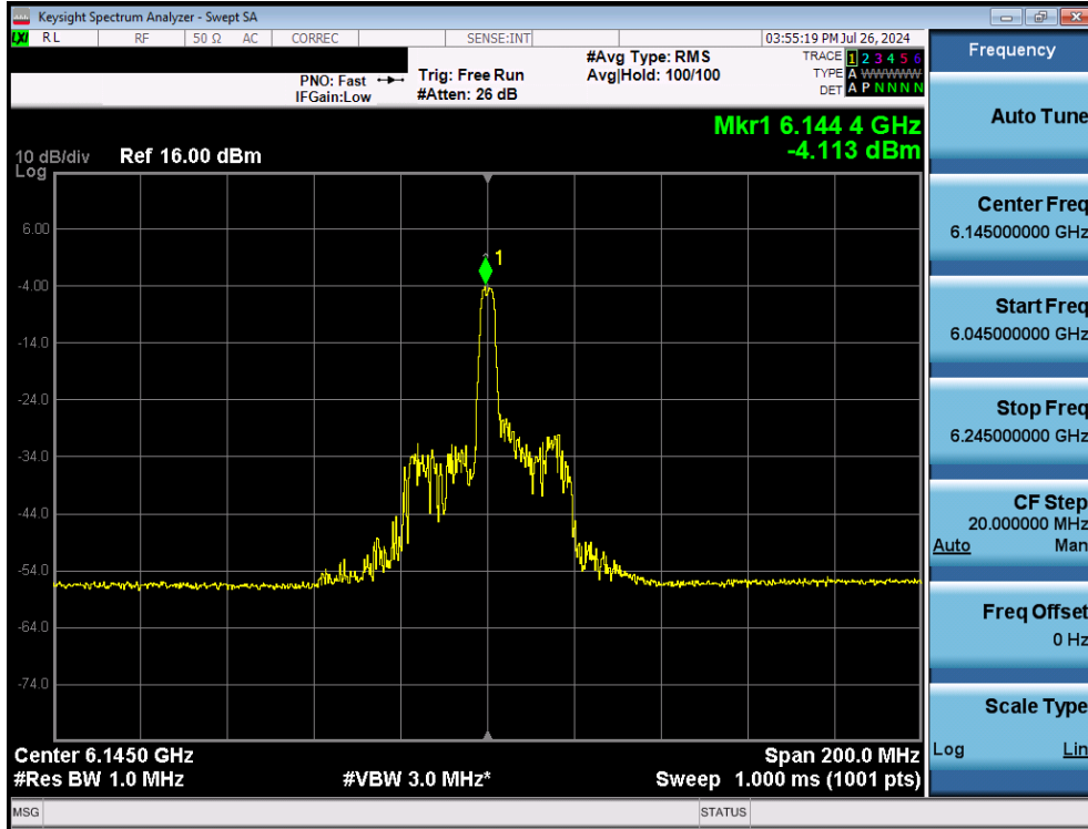
Plot 7-115. Power Spectral Density Plot MIMO ANT1 (80MHz BW 802.11ax/be (26 Tones) (UNII Band 5) – Ch. 39)
