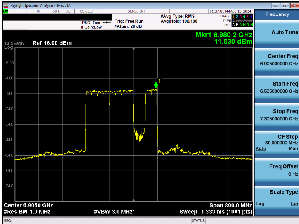
Plot 7-168. Power Spectral Density MIMO ANT1 (320MHz BW 802.11be (2*996+484 Tones) (UNII Band 8) – Ch. 191)
