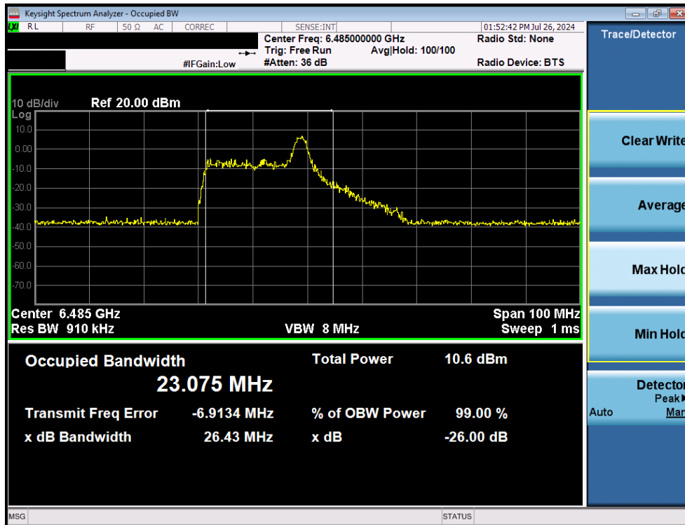
Plot 7-7. Occupied Bandwidth Plot MIMO ANT1 (40MHz BW 802.11ax/be (26 Tones) (UNII Band 6) – Ch. 107)
