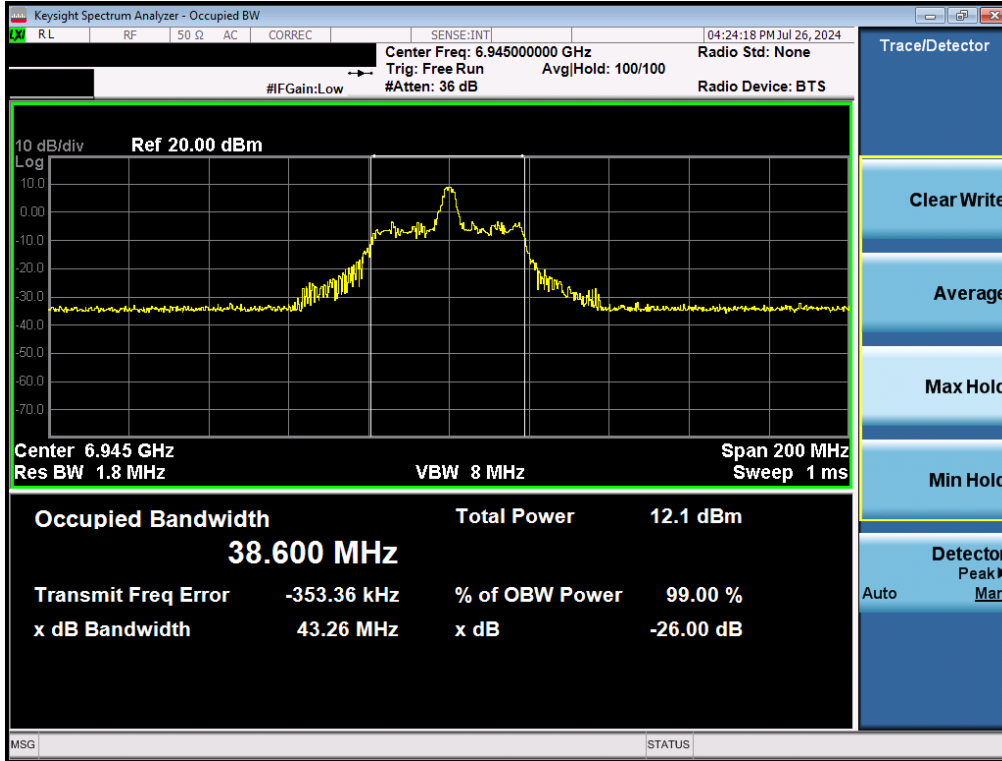
Plot 7-18. Occupied Bandwidth Plot MIMO ANT1 (80MHz BW 802.11ax/be (26 Tones) (UNII Band 8) – Ch. 199)
