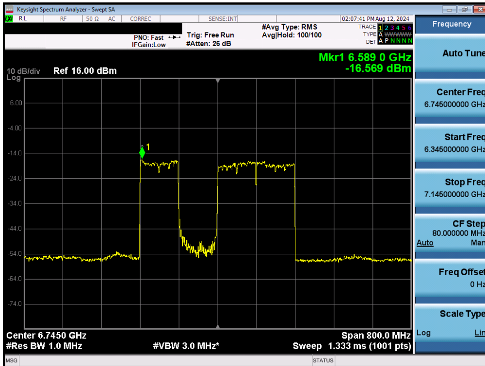
Plot 7-133. Power Spectral Density Plot MIMO ANT2 (320MHz 802.11be (UNII Band 7) – Ch. 159) – LPI/SP-80MHz Punctured
