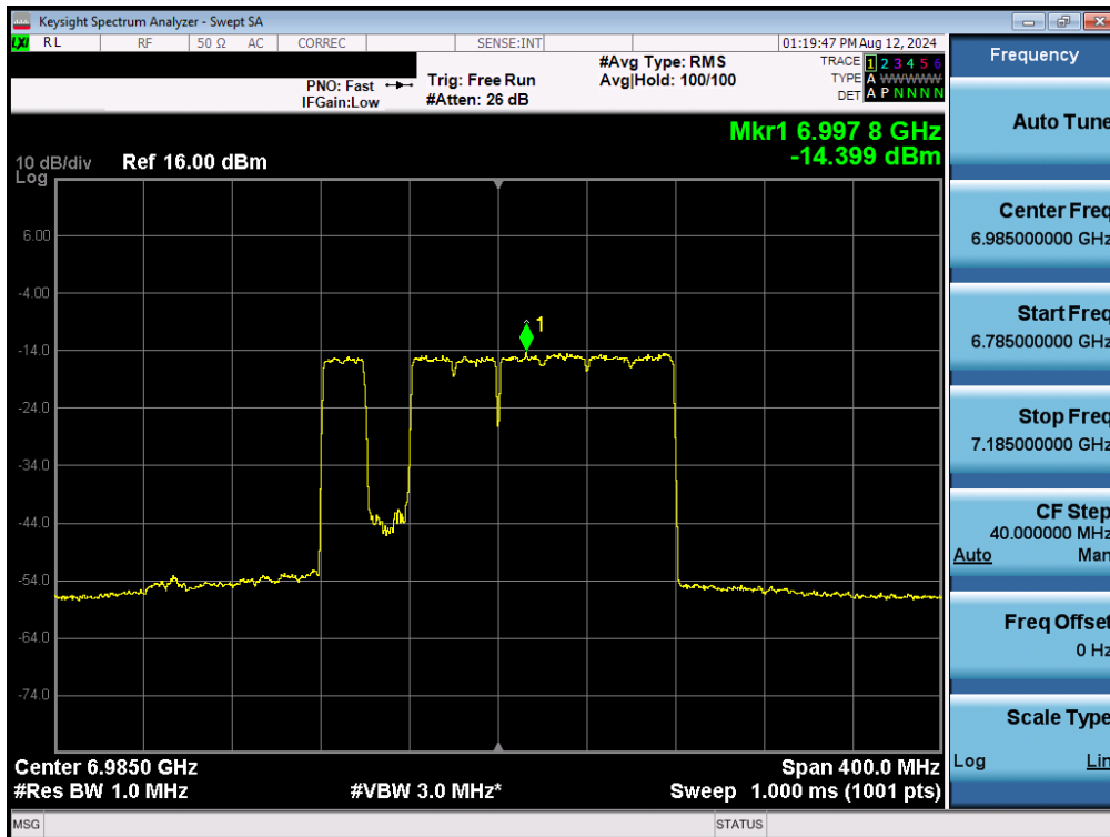
Plot 7-106. Power Spectral Density Plot MIMO ANT1 (160MHz 802.11be (UNII Band 8) – Ch. 207) – LPI - 20MHz Punctured
