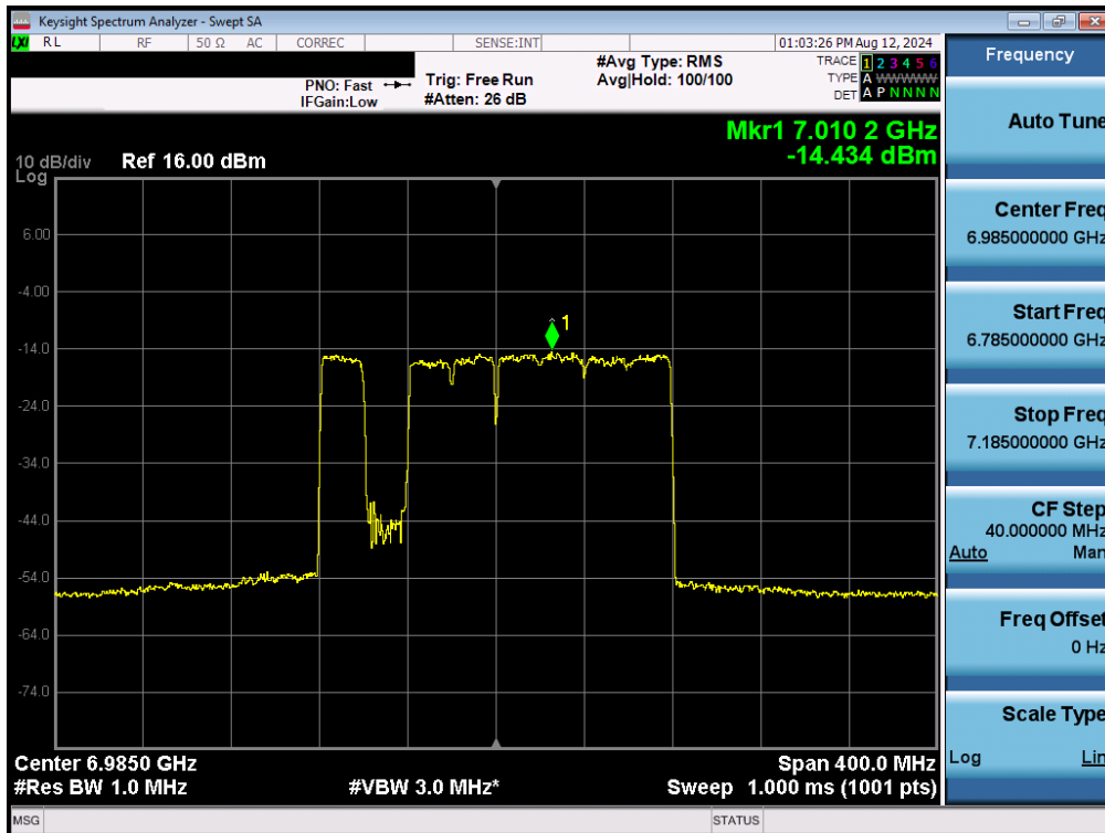
Plot 7-141. Power Spectral Density Plot MIMO ANT1 (160MHz 802.11be (UNII Band 8) – Ch. 207) – LPI - 20MHz Punctured
