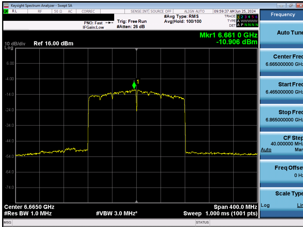
Plot 7-95. Power Spectral Density MIMO ANT1 (160MHz 802.11be (UNII Band 7) – Ch. 143) - LPI/SP
