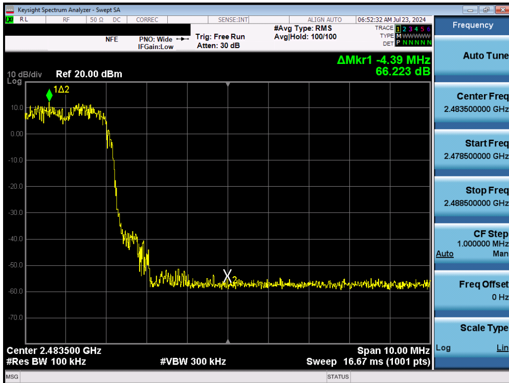
Plot 7-62. Band Edge Plot (Bluetooth with Hopping Enabled, 3 Mbps) – Ant2
