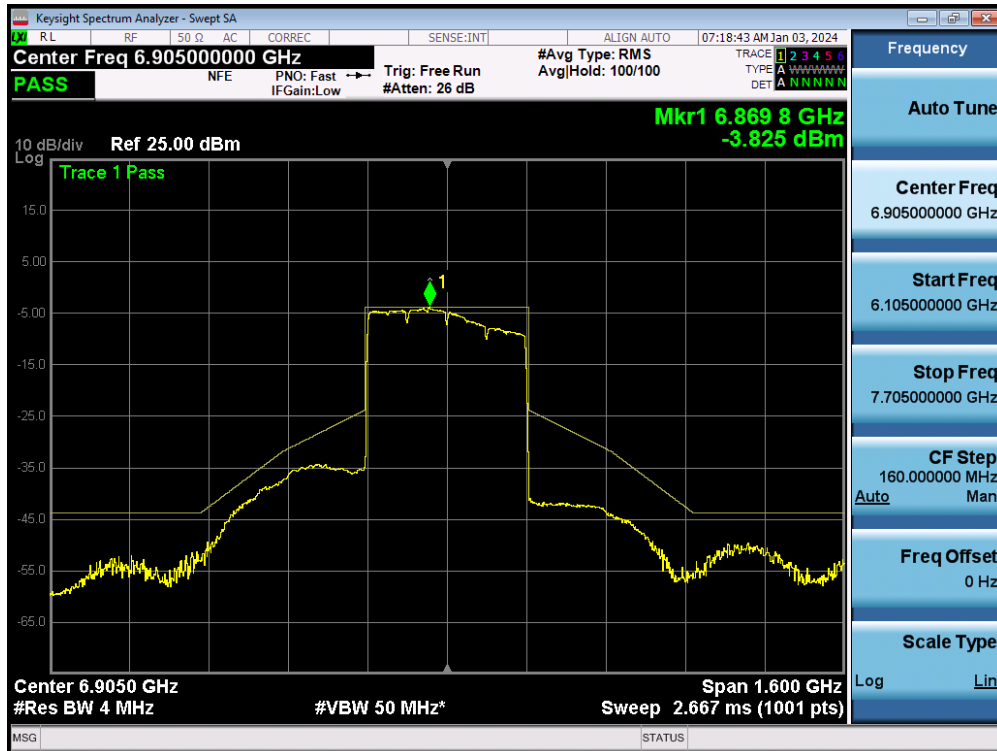
Plot 7-94. In-Band Emission Plot MIMO ANT1 (320MHz BW 802.11be (Full Tone) (UNII Band 7/8) – Ch. 191)
