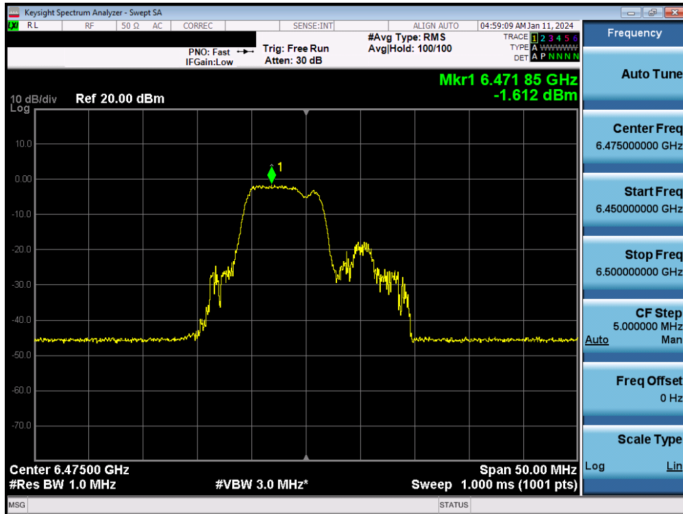
Plot 7-26. Power Spectral Density Plot MIMO ANT1 (20MHz BW 802.11be (52+26 Tone) (UNII Band 6) – Ch. 105)
