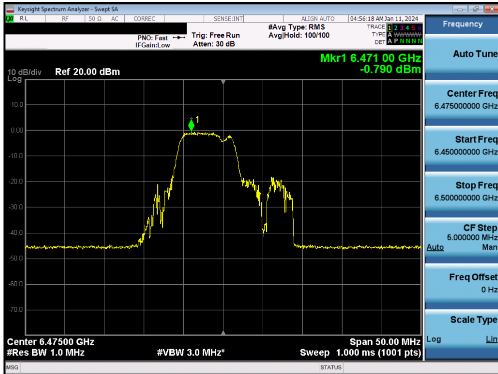
Plot 7-45. Power Spectral Density Plot MIMO ANT2 (20MHz BW 802.11be (52+26 Tone) (UNII Band 6) – Ch. 105)
