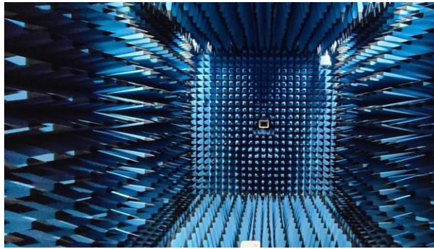
Figure 2: Geometry of Anechoic Chamber for Radiation patterns.
