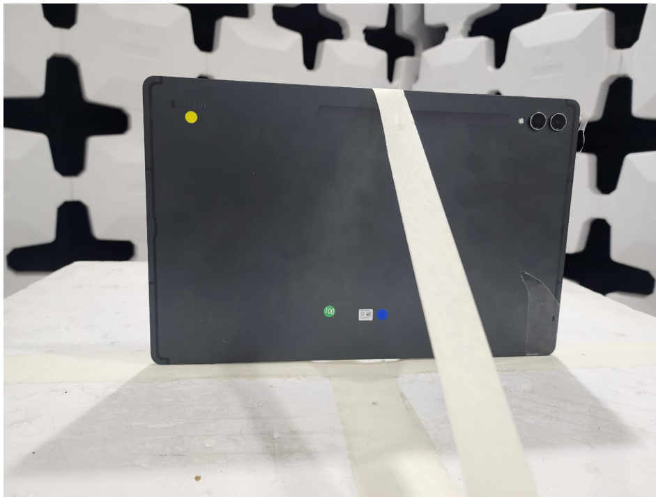
Figure 4. Test Setup – Y Position – 1GHz-18GHz
