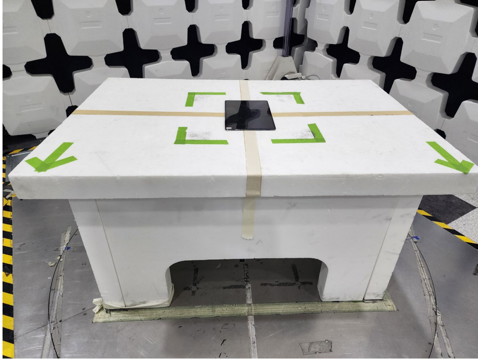
Figure 7. Test Setup – X Position – 30MHz-1GHz
