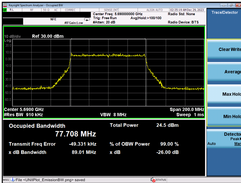
Plot 7-10. 26dB Bandwidth Plot MIMO ANT1 (80MHz BW 802.11be (UNII Band 2C) – Ch. 138)
