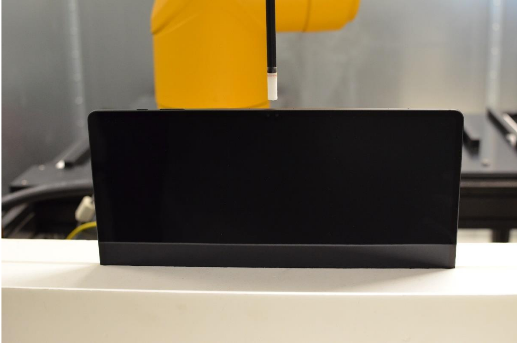
Figure G-29 Near Field Power Density Test Setup Photo – Tablet, Right edge at 7mm – WIFI MIMO
