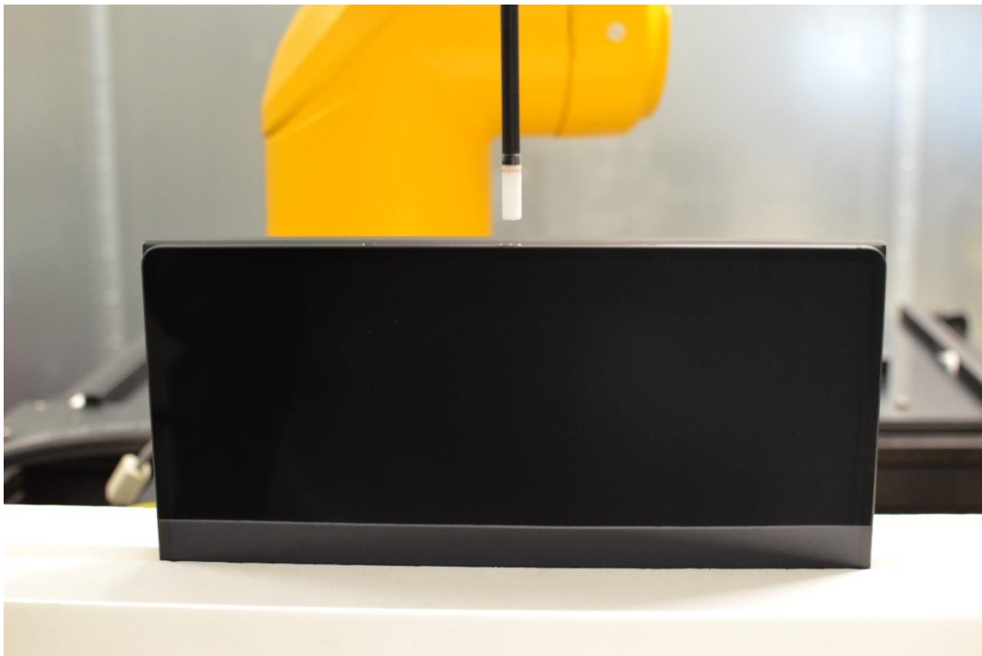
Figure G-32 Near Field Power Density Test Setup Photo – Tablet, Left edge at 9mm with Keyboard (Variant 1) – WIFI MIMO
