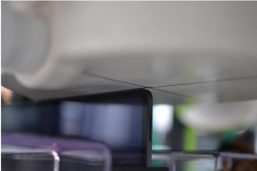
Figure G-17 SAR Test Setup Photo – Tablet, Left Edge at 0mm – WIFI MIMO
