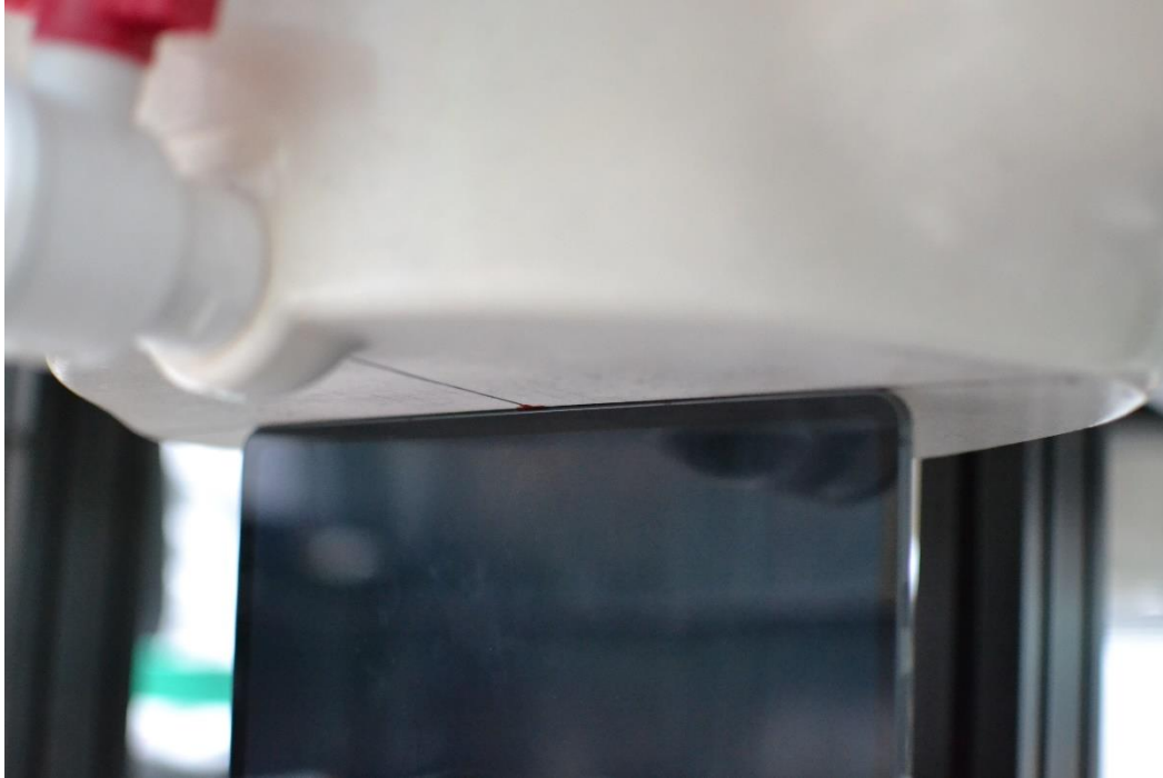
Figure G-13 SAR Test Setup Photo – Tablet, Top Edge at 0mm – WIFI MIMO
