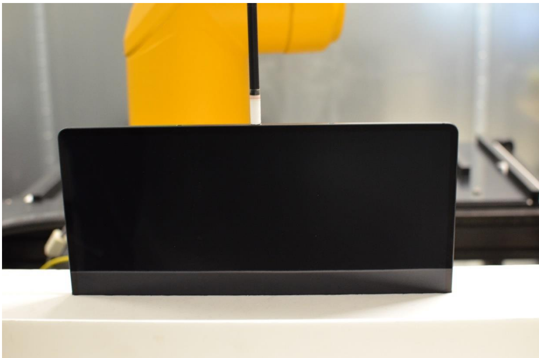
Figure G-30 Near Field Power Density Test Setup Photo – Tablet, Left edge at 2mm – WIFI MIMO
