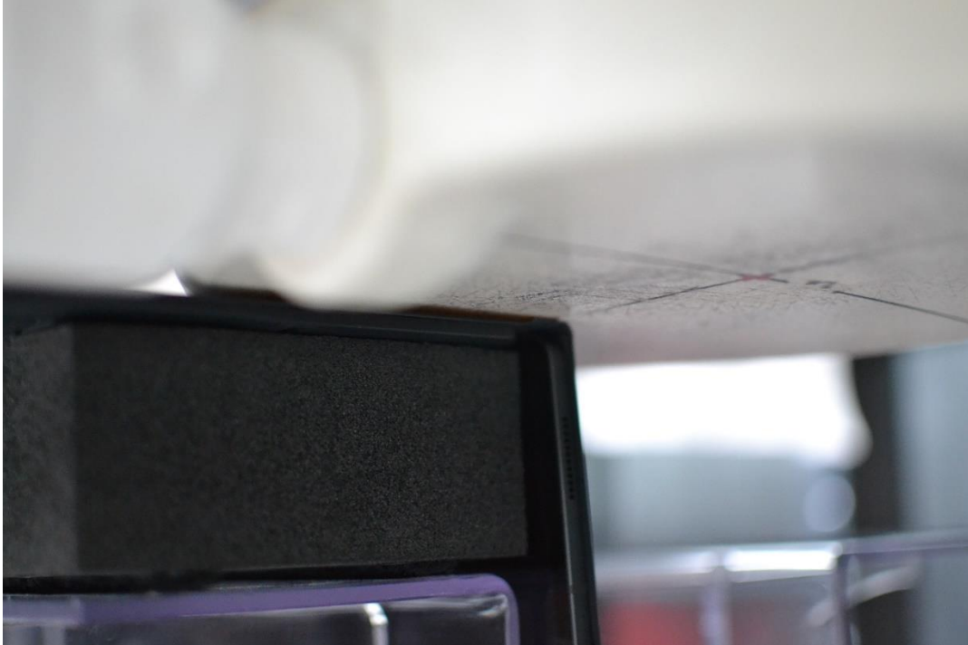
Figure G-19 SAR Test Setup Photo – Laptop, Bottom Edge with Keyboard (Variant 1) at 0mm – WIFI MIMO
