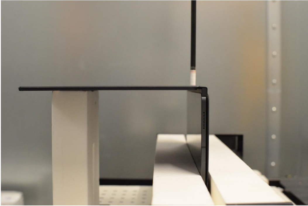
Figure G-35 Near Field Power Density Test Setup Photo – Laptop, Bottom edge at 2mm with Keyboard (Variant 2) – WIFI MIMO
