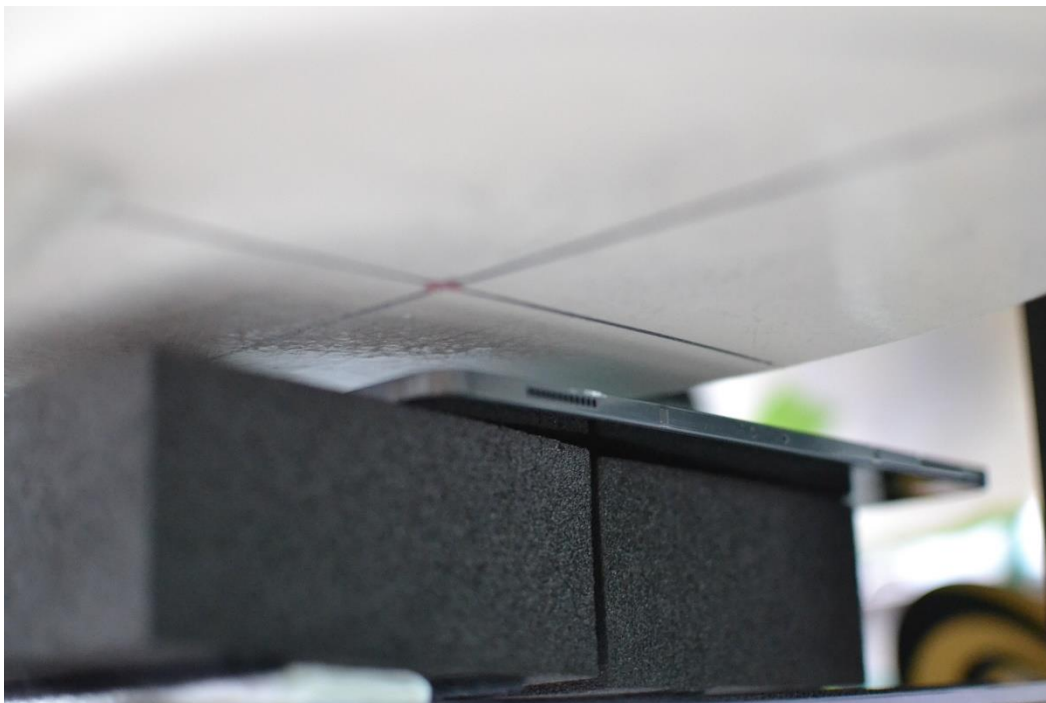
Figure G-6 SAR Test Setup Photo – Tablet, Back side at 15mm – WIFI MIMO (Peak 2)
