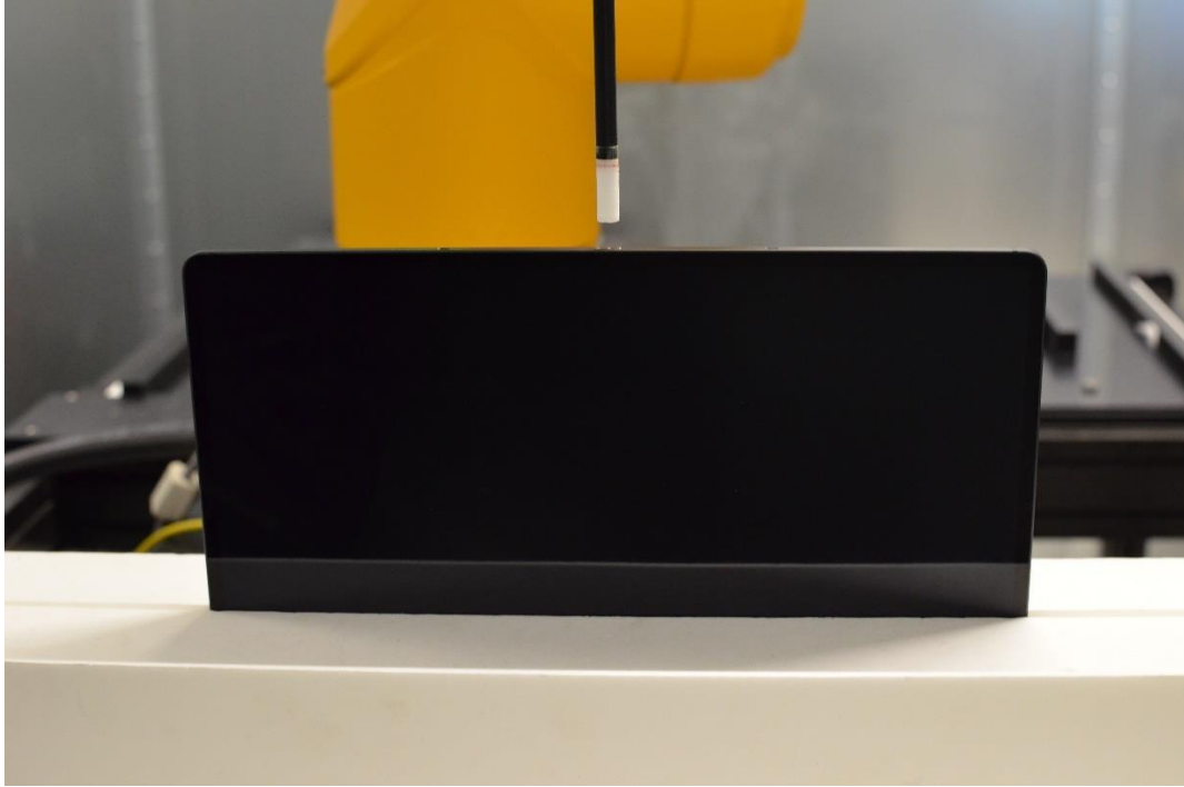
Figure G-31 Near Field Power Density Test Setup Photo – Tablet, Left edge at 9mm – WIFI MIMO
