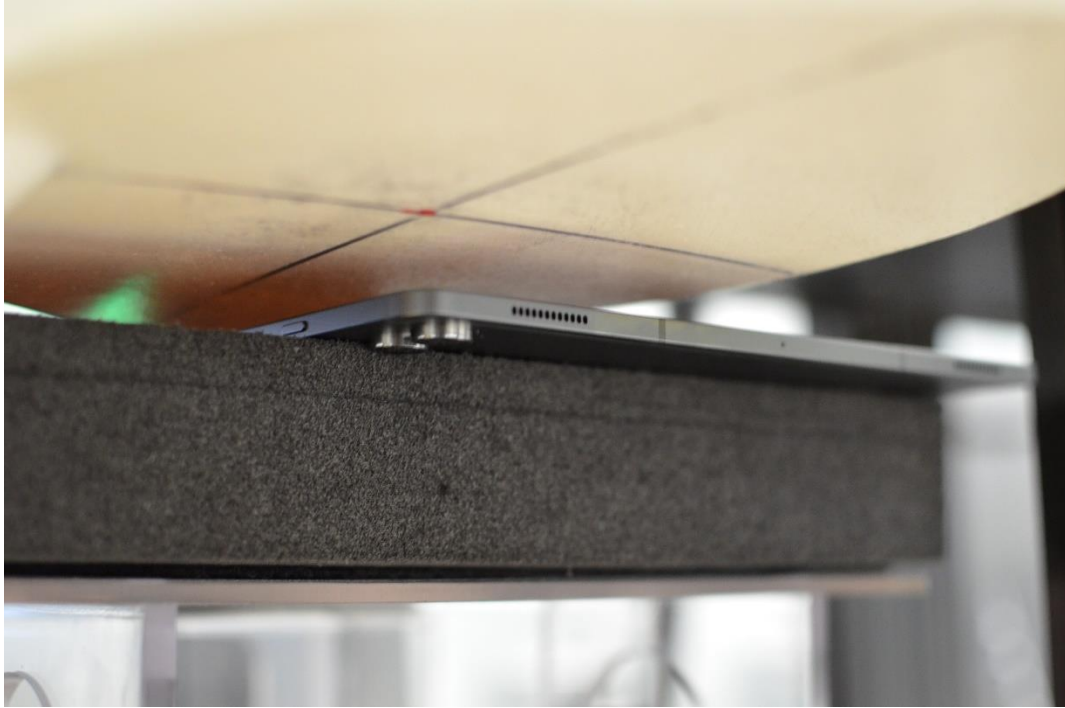
Figure G-11 SAR Test Setup Photo – Tablet, Front side at 15mm – WIFI MIMO (Peak 1)
