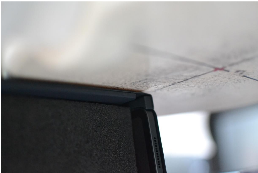
Figure G-20 SAR Test Setup Photo – Laptop, Bottom Edge with Keyboard (Variant 2) at 0mm – WIFI MIMO
