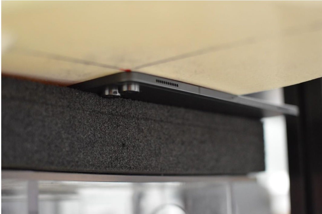
Figure G-9 SAR Test Setup Photo – Tablet, Front side at 0mm – WIFI MIMO (Peak 1)
