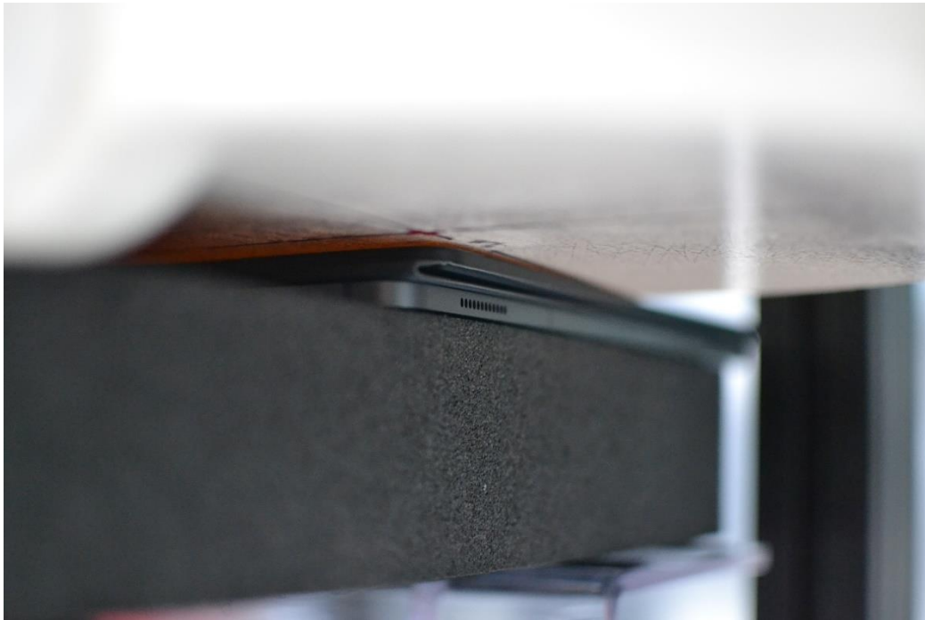
SAR Test Setup Photo 6 – Back side with Keyboard (Variant 1) at 0mm for WIFI/BT Antenna 2 and WIFI MIMO (Peak 2)
