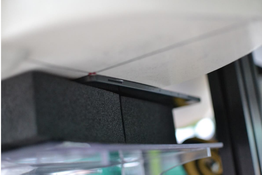
SAR Test Setup Photo 5 – Back side at 0mm for WIFI/BT Antenna 2 and WIFI MIMO (Peak 2)
