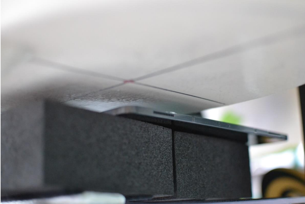
SAR Test Setup Photo 3 – Back side at 15mm for WIFI/BT Antenna 2 and WIFI MIMO (Peak 2)
