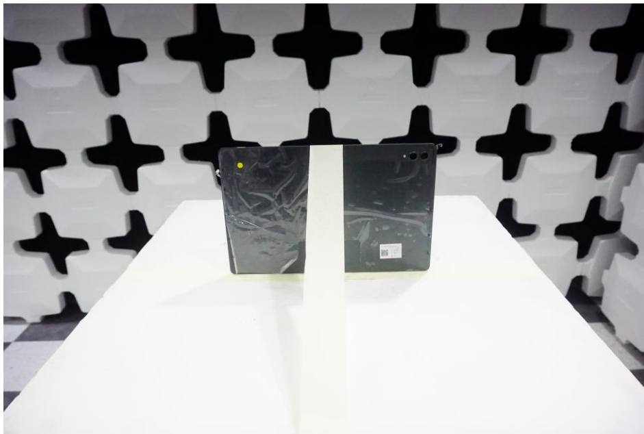
Figure 6. Test Setup – Y Position – 1GHz-18GHz
