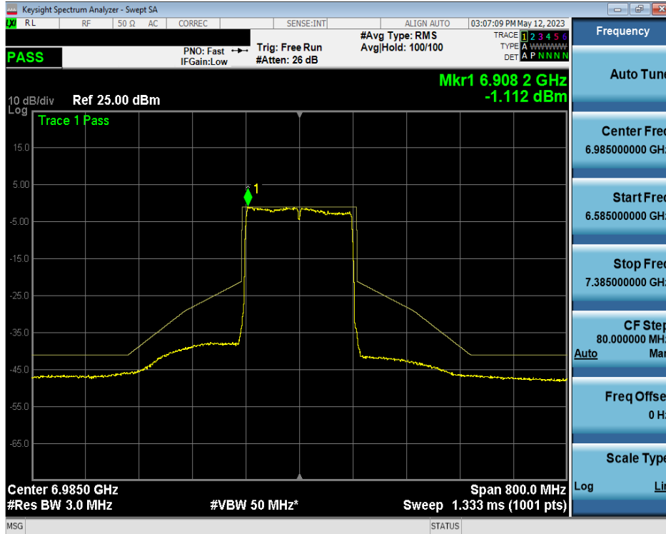
Plot 7-480. In-Band Emission Plot MIMO ANT2 (160MHz BW 802.11ax (Full Tone) (UNII Band 8) – Ch. 207)
