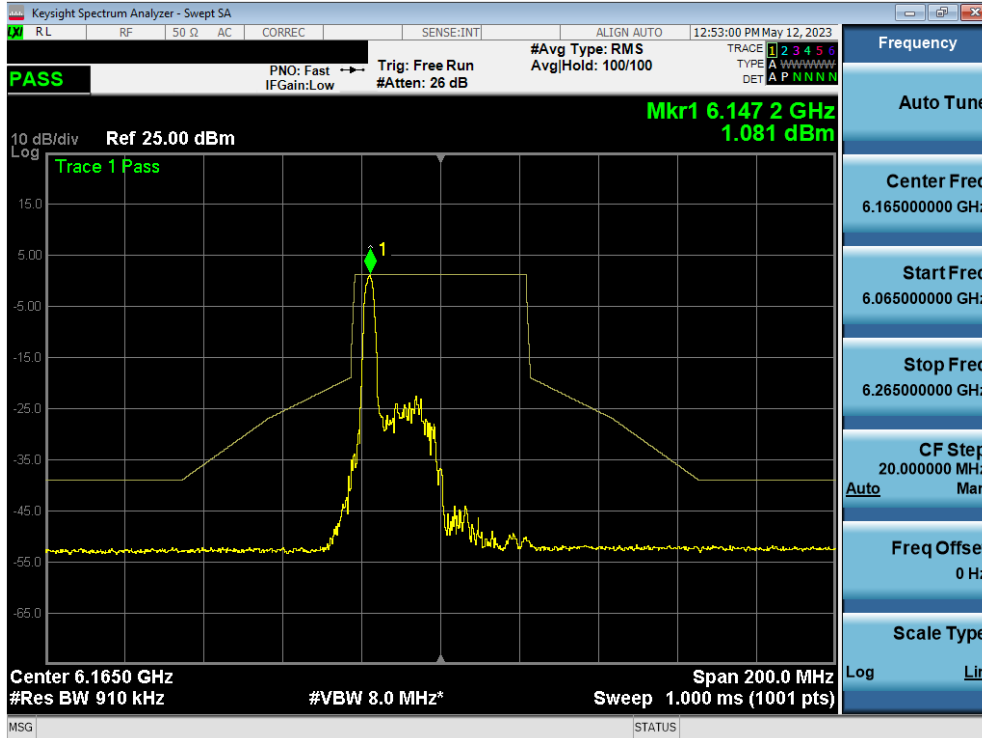
Plot 7-325. In-Band Emission Plot MIMO ANT1 (40MHz BW 802.11ax (26 Tones) (UNII Band 5) – Ch. 43)
