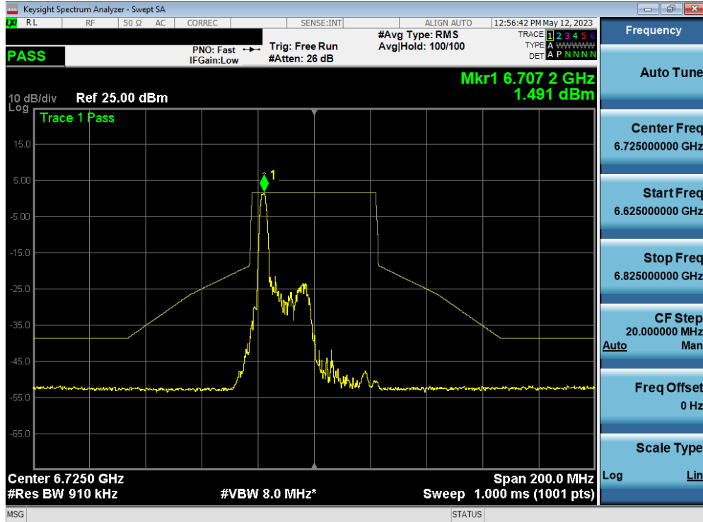
Plot 7-345. In-Band Emission Plot MIMO ANT1 (40MHz BW 802.11ax (26 Tones) (UNII Band 7) – Ch. 155)
