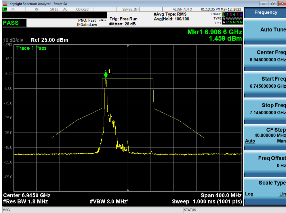
Plot 7-358. In-Band Emission Plot MIMO ANT1 (80MHz BW 802.11ax (26 Tones) (UNII Band 8) – Ch. 199)
