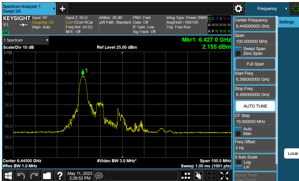
Plot 7-256. Power Spectral Density Plot MIMO ANT2 (40MHz BW 802.11ax (26 Tones) (UNII Band 6) – Ch. 99)
