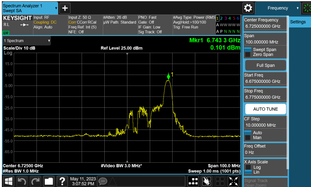
Plot 7-265. Power Spectral Density Plot MIMO ANT2 (40MHz BW 802.11ax (26 Tones) (UNII Band 7) – Ch. 155)
