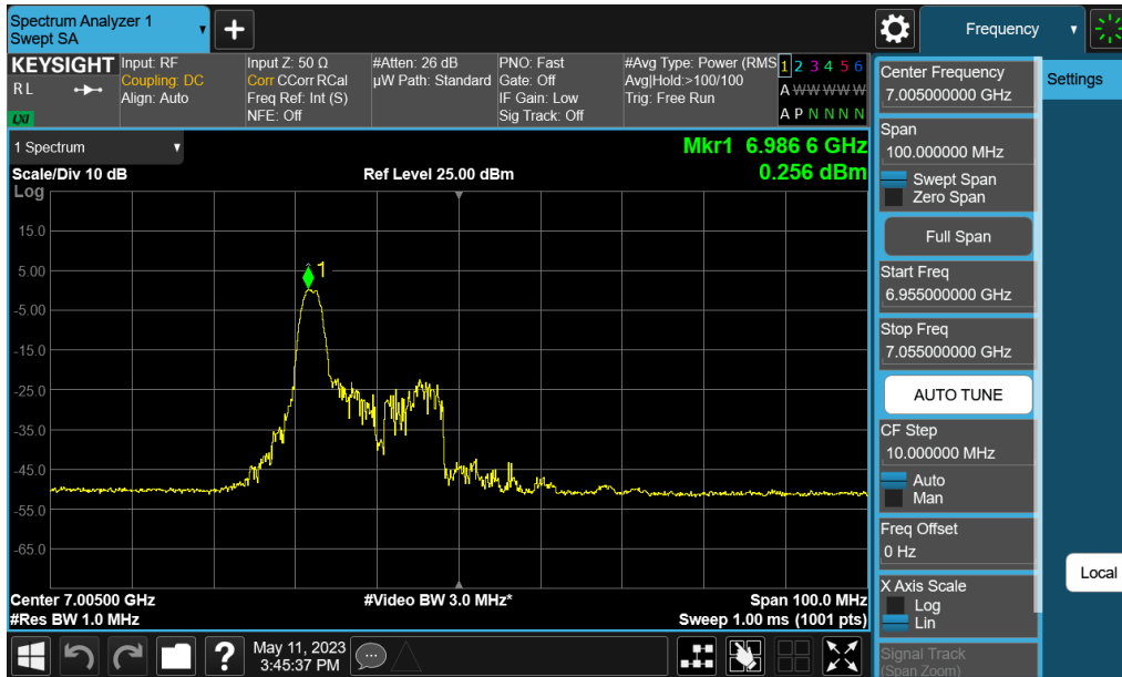
Plot 7-276. Power Spectral Density Plot MIMO ANT2 (40MHz BW 802.11ax (26 Tones) (UNII Band 8) – Ch. 211)
