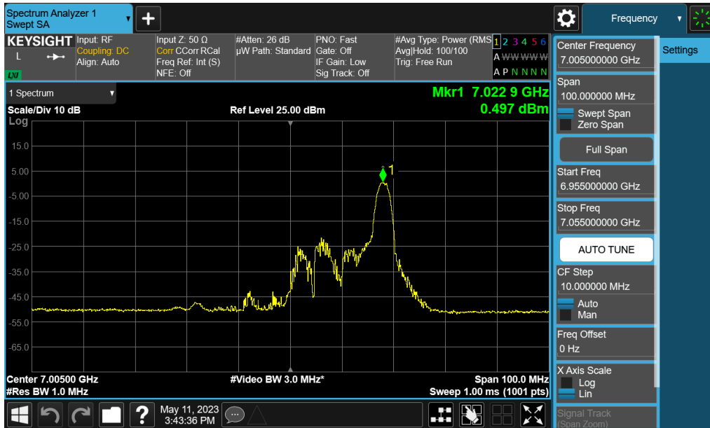
Plot 7-196. Power Spectral Density Plot MIMO ANT1 (40MHz BW 802.11ax (26 Tones) (UNII Band 8) – Ch. 211)
