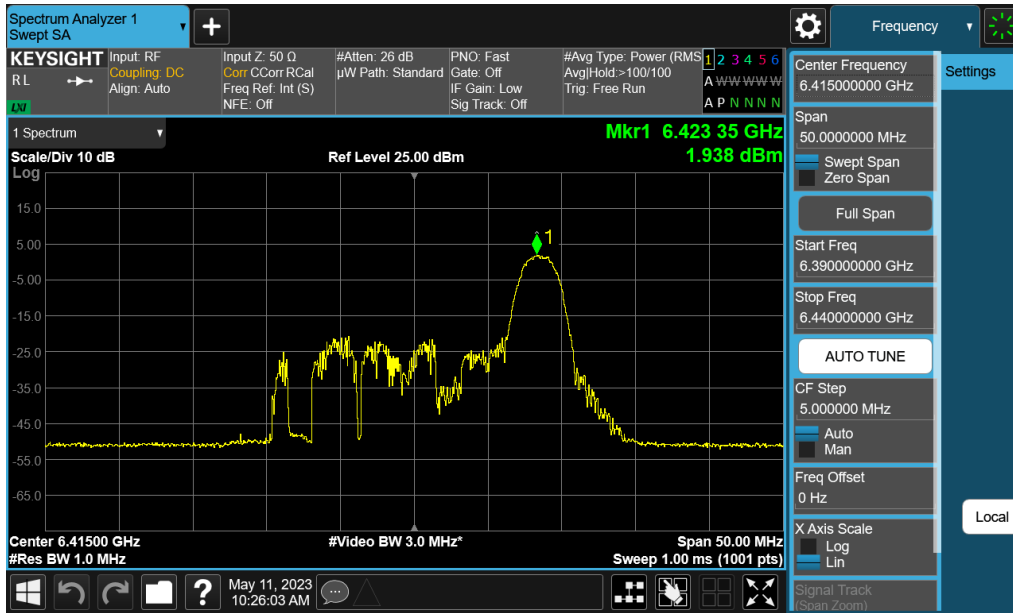
Plot 7-243. Power Spectral Density Plot MIMO ANT2 (20MHz BW 802.11ax (26 Tones) UNII Band 5) – Ch. 93)
