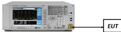
Figure 7-3. Test Instrument & Measurement Setup
