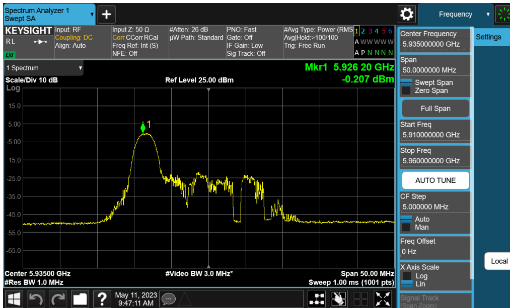
Plot 7-161. Power Spectral Density Plot MIMO ANT1 (20MHz BW 802.11ax (26 Tones) UNII Band 5) – Ch. 2
