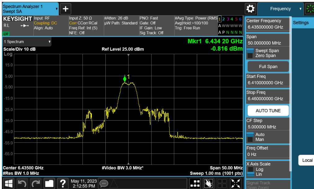
Plot 7-173. Power Spectral Density Plot MIMO ANT1 (20MHz BW 802.11ax (26 Tones) (UNII Band 6) – Ch. 97)
