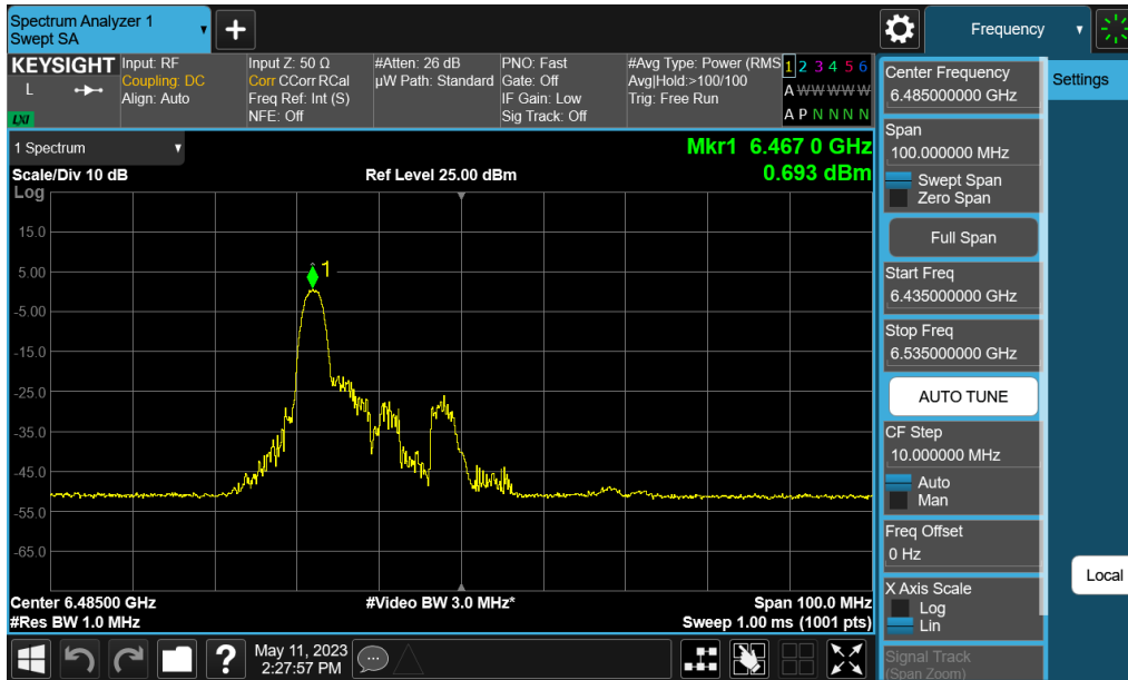
Plot 7-177. Power Spectral Density Plot MIMO ANT1 (40MHz BW 802.11ax (26 Tones) (UNII Band 6) – Ch. 107)
