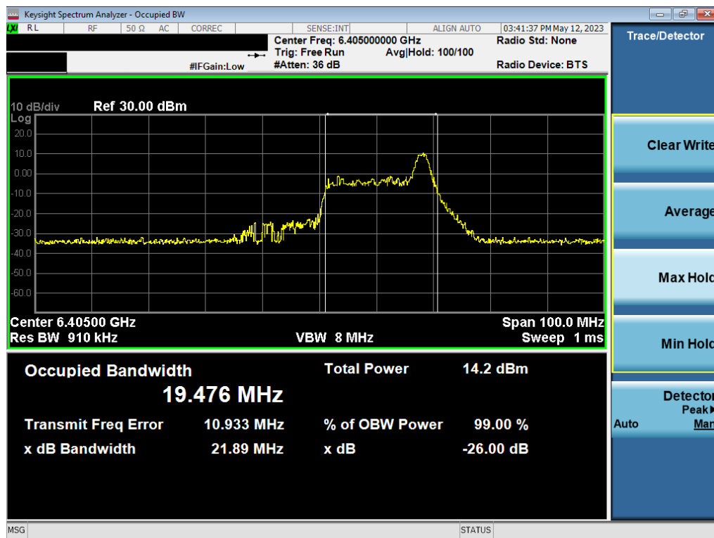
Plot 7-86. Occupied Bandwidth Plot MIMO ANT2 (40MHz BW 802.11ax (26 Tones) (UNII Band 5) – Ch. 91)
