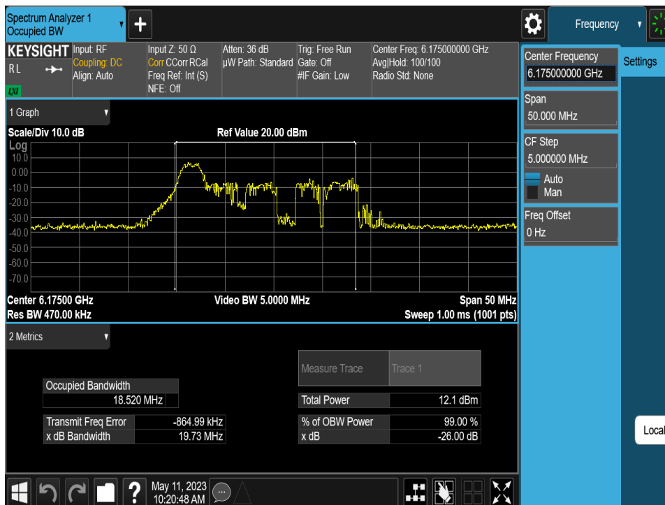
Plot 7-82. Occupied Bandwidth Plot MIMO ANT2 (20MHz BW 802.11ax (26 Tones) (UNII Band 5) – Ch. 45)
