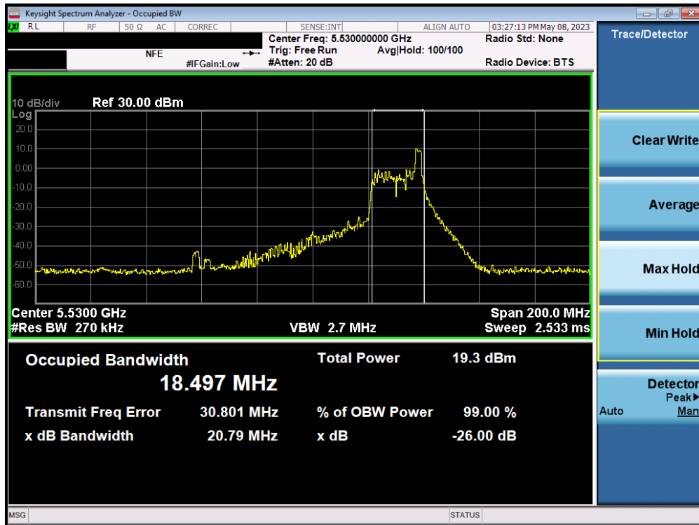
Plot 7-69. 26dB Bandwidth Plot MIMO ANT2 (80MHz BW 802.11ax – 26 Tones (UNII Band 2C) – Ch. 106)
