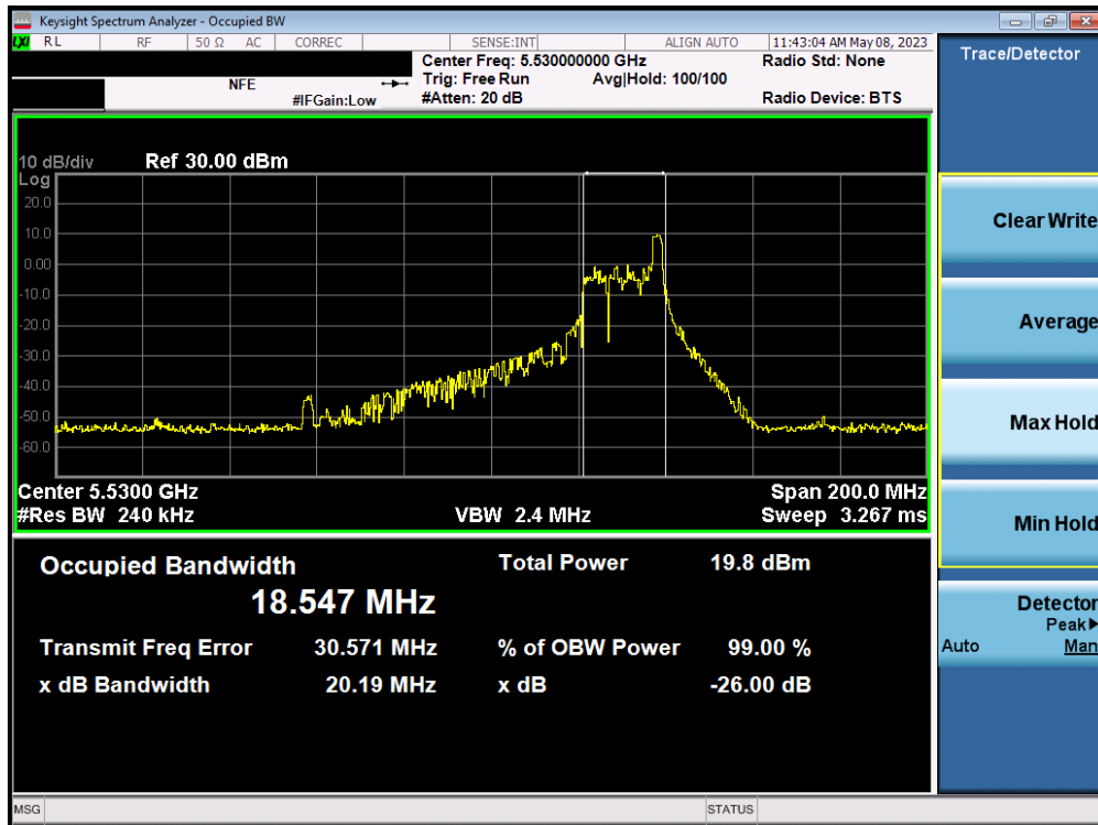
Plot 7-21. 26dB Bandwidth Plot MIMO ANT1 (80MHz BW 802.11ax – 26 Tones (UNII Band 2C) – Ch. 106)
