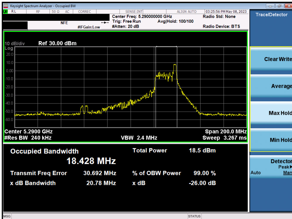
Plot 7-14. 26dB Bandwidth Plot MIMO ANT1 (80MHz BW 802.11ax – 26 Tones (UNII Band 2A) – Ch. 58)
