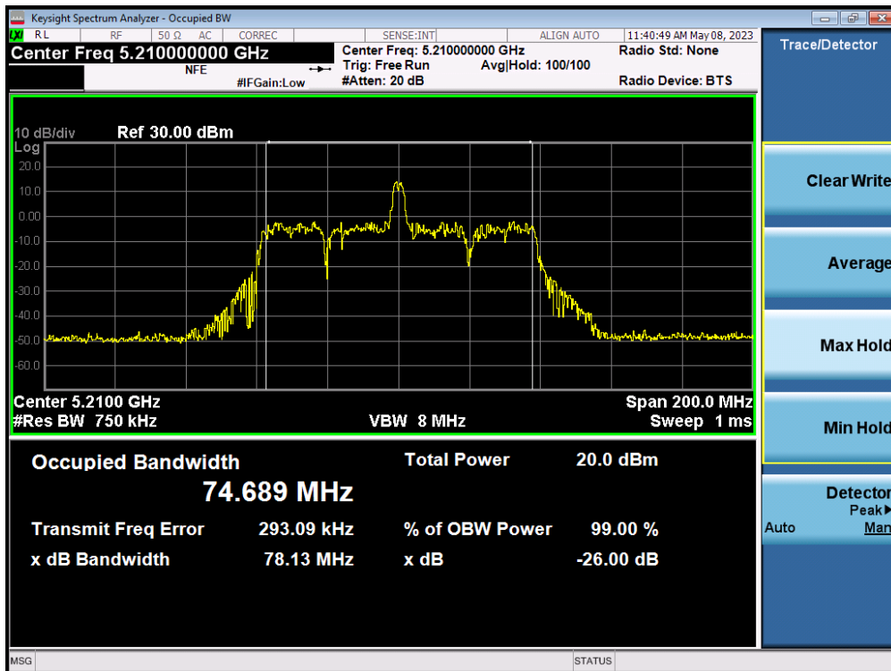
Plot 7-6. 26dB Bandwidth Plot MIMO ANT1 (80MHz BW 802.11ax – 26 Tones (UNII Band 1) – Ch. 42)
