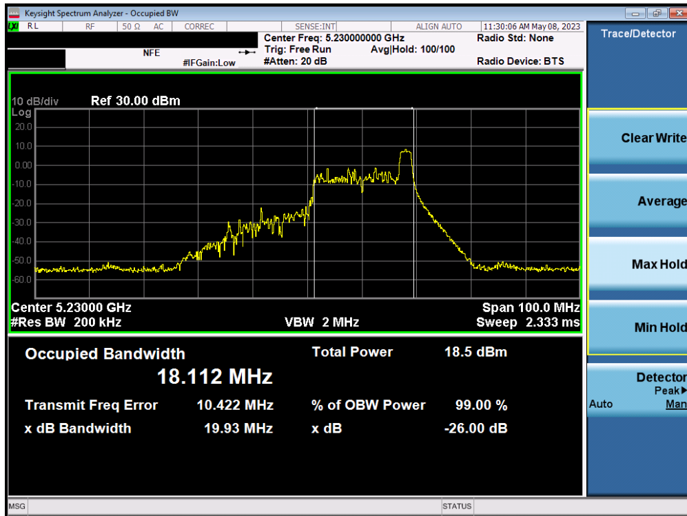
Plot 7-5. 26dB Bandwidth Plot MIMO ANT1 (40MHz BW 802.11ax – 26 Tones (UNII Band 1) – Ch. 46)
