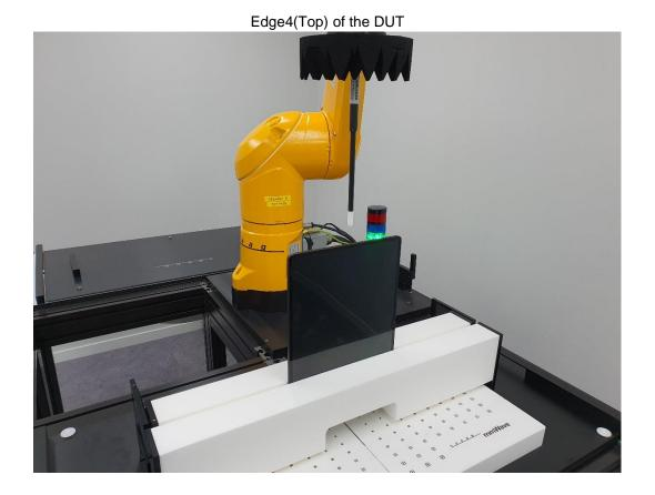
**SAR test Setup Photo**
