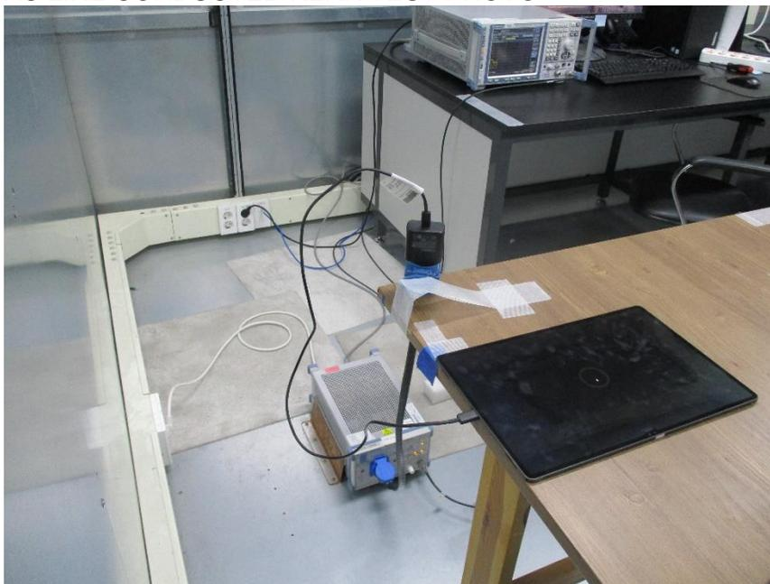
6) **AC LINE CONDUCTED MEASUREMENT SETUP(S-pen WPT)**
