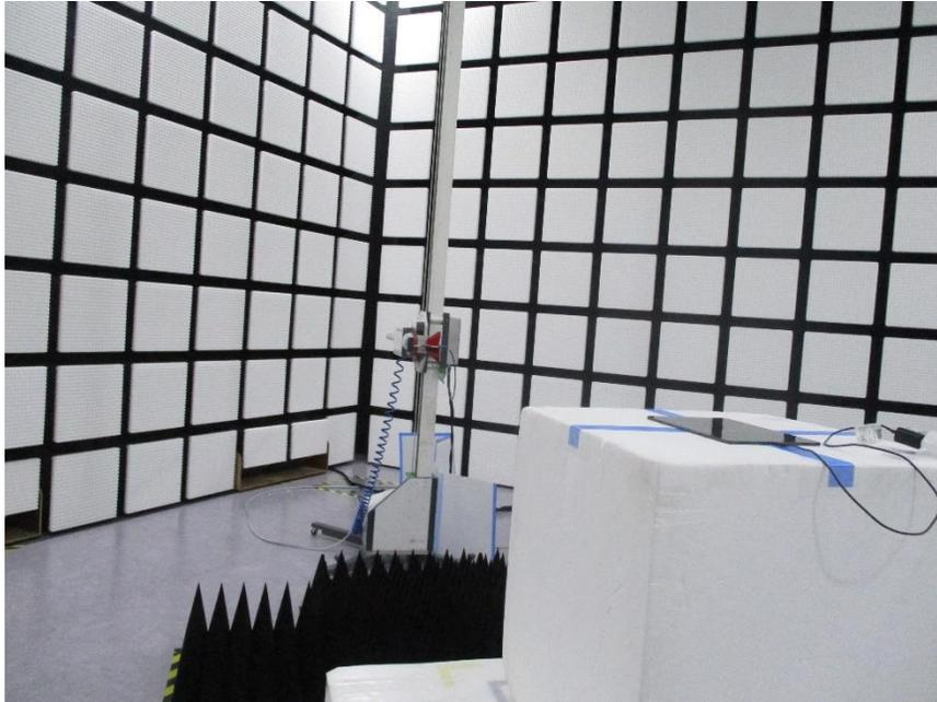
3) RADIATED RF MEASUREMENT SETUP (WPT)
