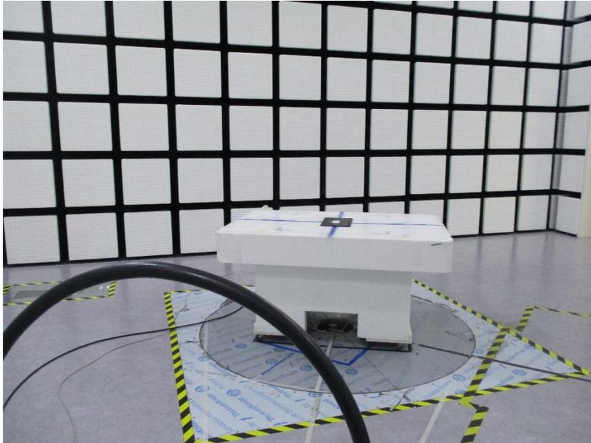
4) RADIATED RF MEASUREMENT SET-UP (Axis)
