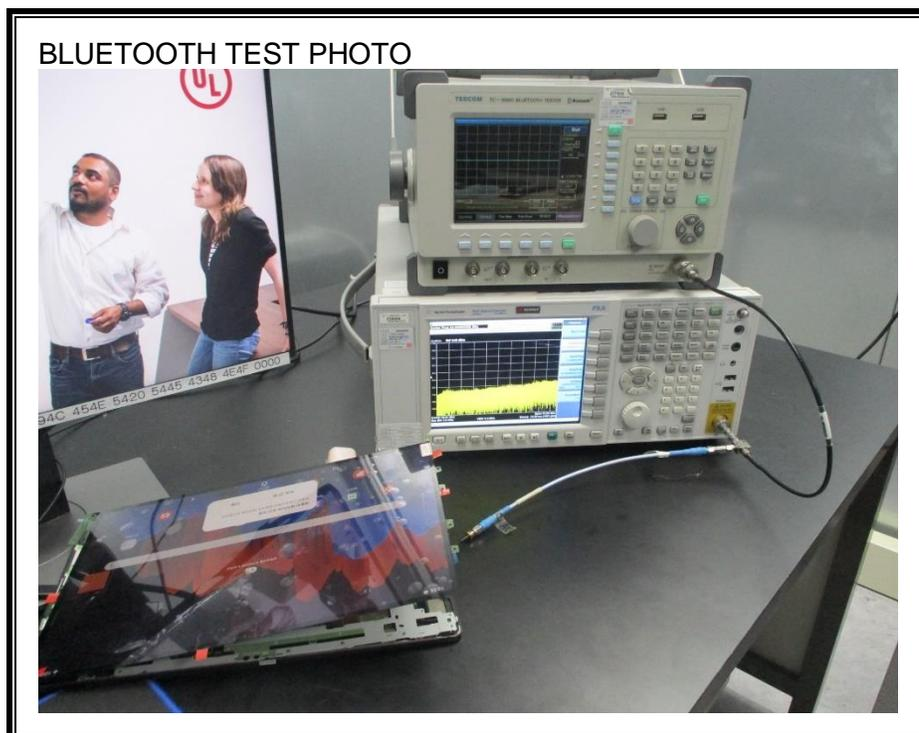
3) CONDUCTED RF MEASUREMENT SETUP (DFS)
