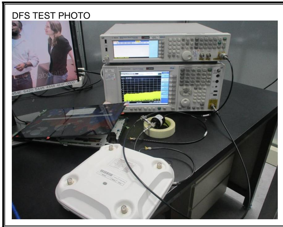
4) CONDUCTED RF MEASUREMENT SETUP (CBP)
