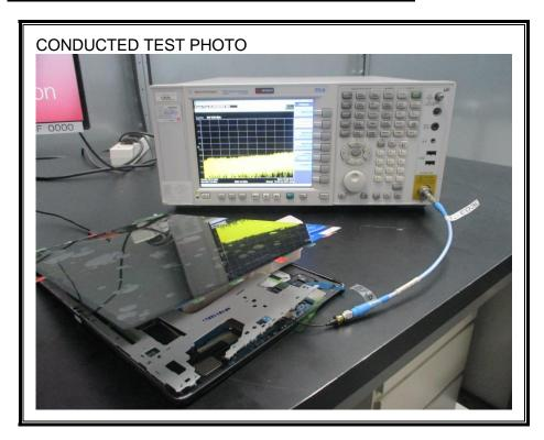
2) CONDUCTED RF MEASUREMENT SETUP (Bluetooth)
