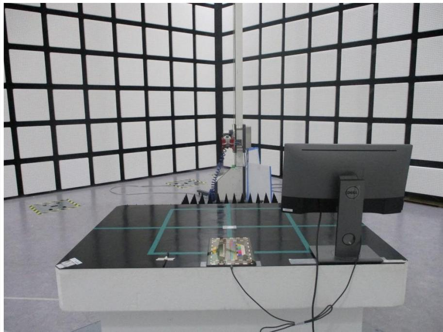
4) Test case 5 : USB Data Communication with PC
