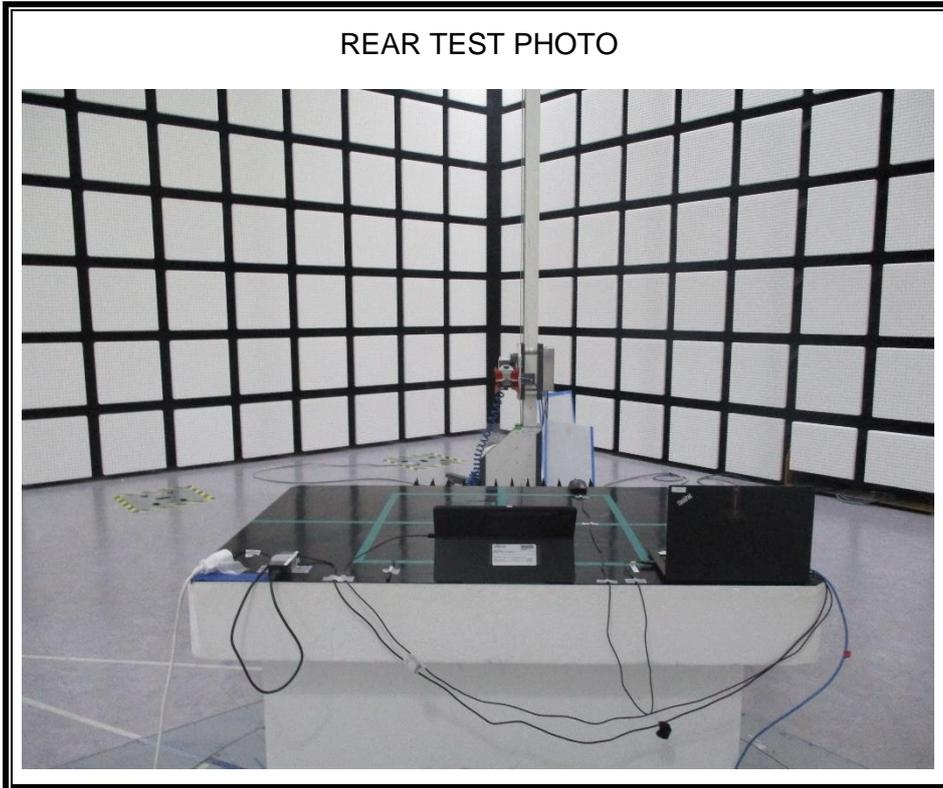
6) Test case 7 : With Keyboard continuous input Key("H" Pattern) + charging
