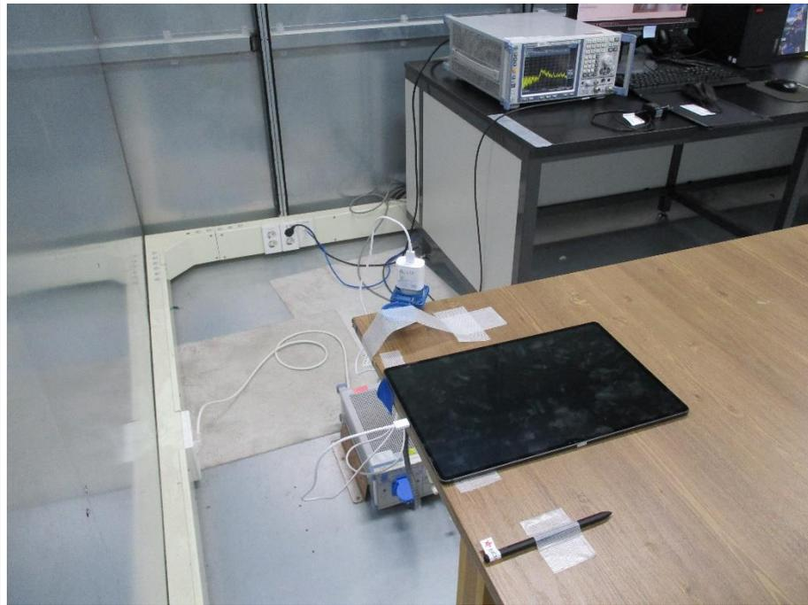
3) Test case 5 : USB Data Communication with PC
