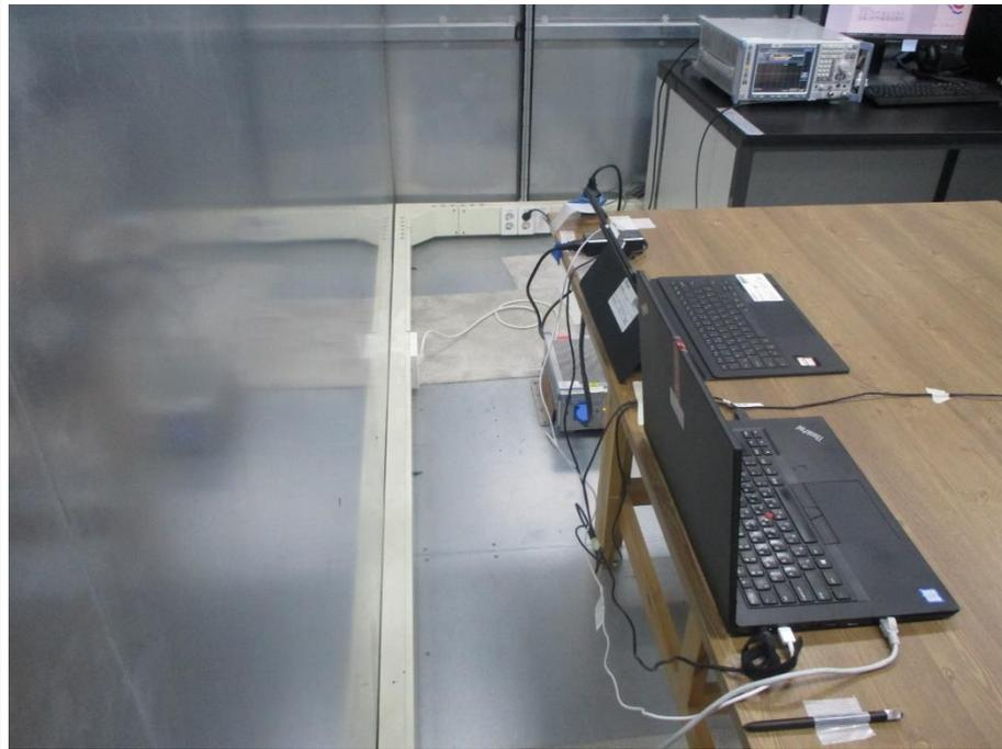
5) **Test case 7 : With Keyboard continuous input Key("H" Pattern) + charging**
