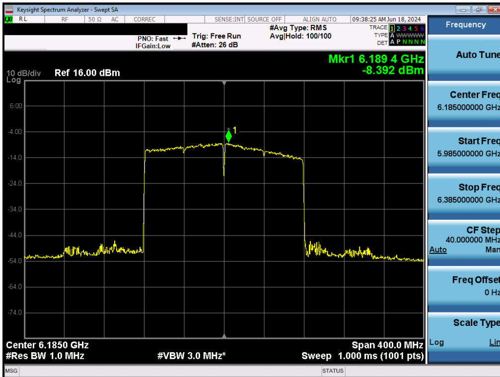
Plot 7-116. Power Spectral Density Plot MIMO ANT2 (160MHz BW 802.11ax (Full Tones) (UNII Band 5) – Ch. 47) - LPI/SP
