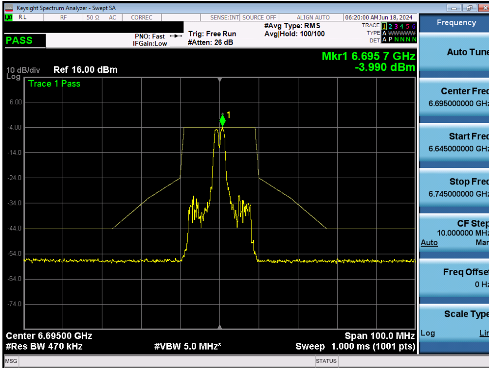
Plot 7-169. In-Band Emissions Plot MIMO ANT2 (20MHz BW 802.11ax (26 Tones) (UNII Band 7) – Ch. 149) - LPI/SP
