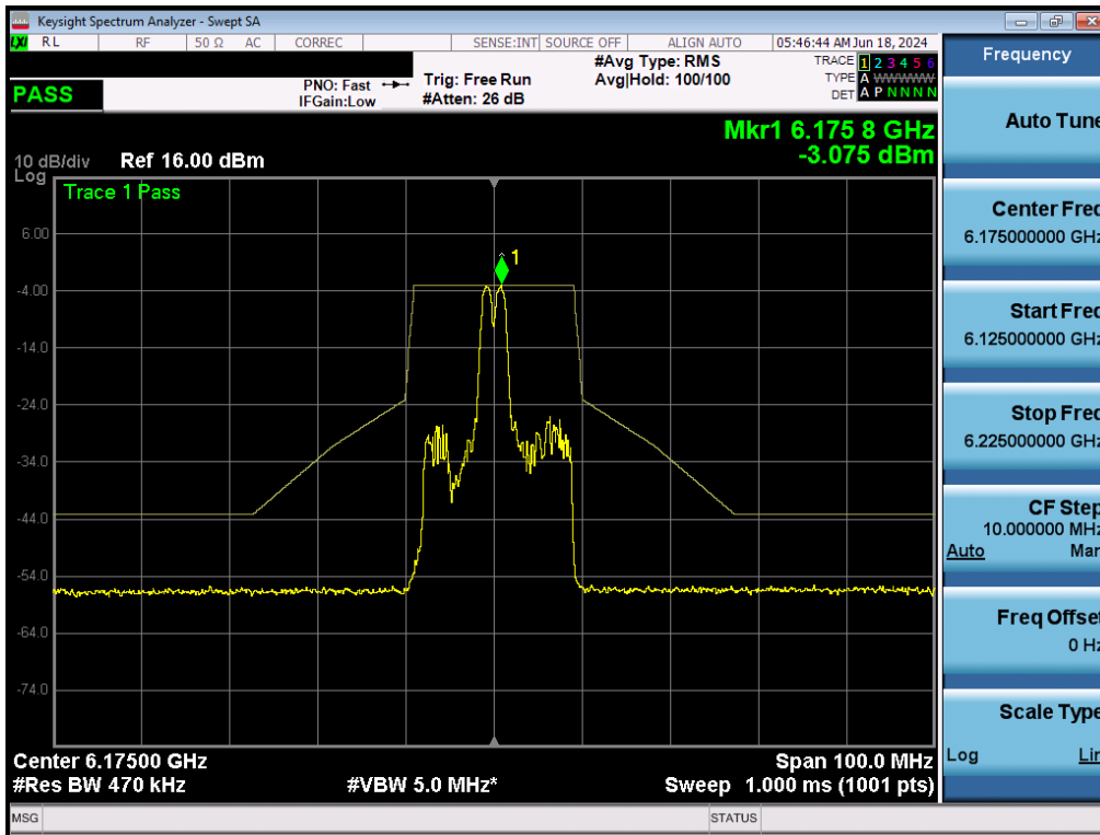
Plot 7-161. In-Band Emissions Plot MIMO ANT2 (20MHz BW 802.11ax (26 Tones) (UNII Band 5) – Ch. 45) - LPI/SP
