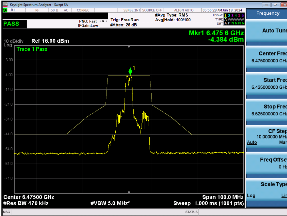
Plot 7-165. In-Band Emissions Plot MIMO ANT2 (20MHz BW 802.11ax (26 Tones) (UNII Band 6) – Ch. 105) - LPI/SP
