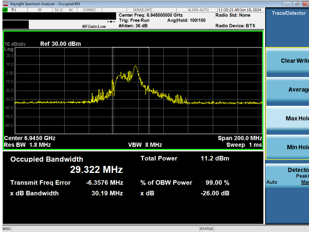
Plot 7-15. Occupied Bandwidth Plot MIMO ANT1 (80MHz BW 802.11ax (26 Tones) (UNII Band 8) – Ch. 199)
