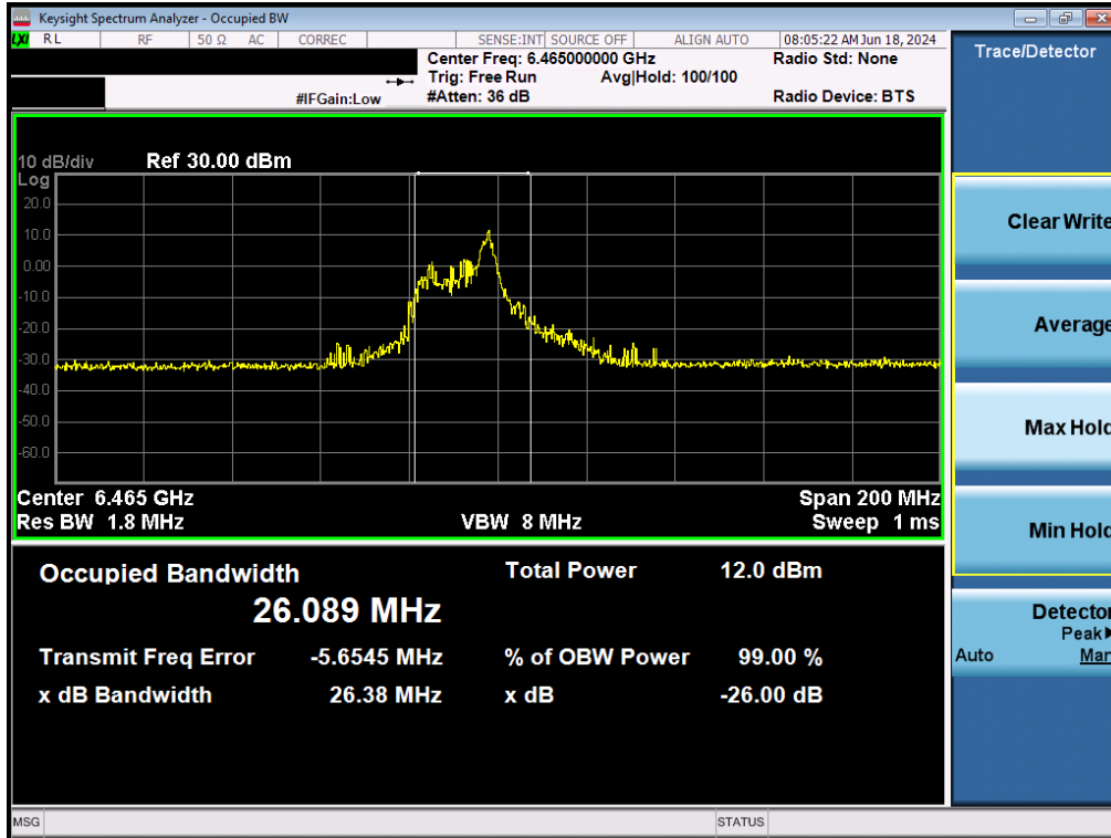
Plot 7-39. Occupied Bandwidth Plot MIMO ANT2 (80MHz BW 802.11ax (26 Tones) (UNII Band 6) – Ch. 103)
