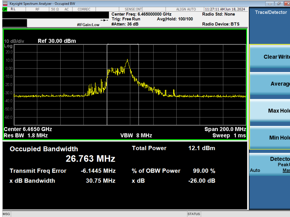
Plot 7-7. Occupied Bandwidth Plot MIMO ANT1 (80MHz BW 802.11ax (26 Tones) (UNII Band 6) – Ch. 103)
