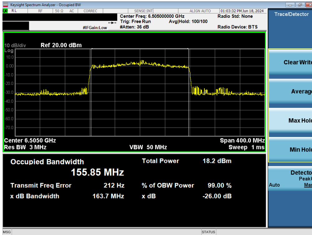
Plot 7-24. Occupied Bandwidth Plot MIMO ANT1 (160MHz BW 802.11ax (Full Tones) (UNII Band 6) – Ch. 111)
