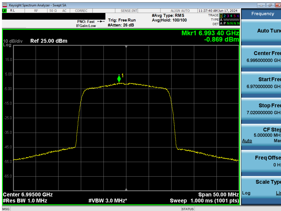
Plot 7-57. Power Spectral Density MIMO ANT1 (20MHz 802.11ax (UNII Band 8) – Ch. 209) - LPI
