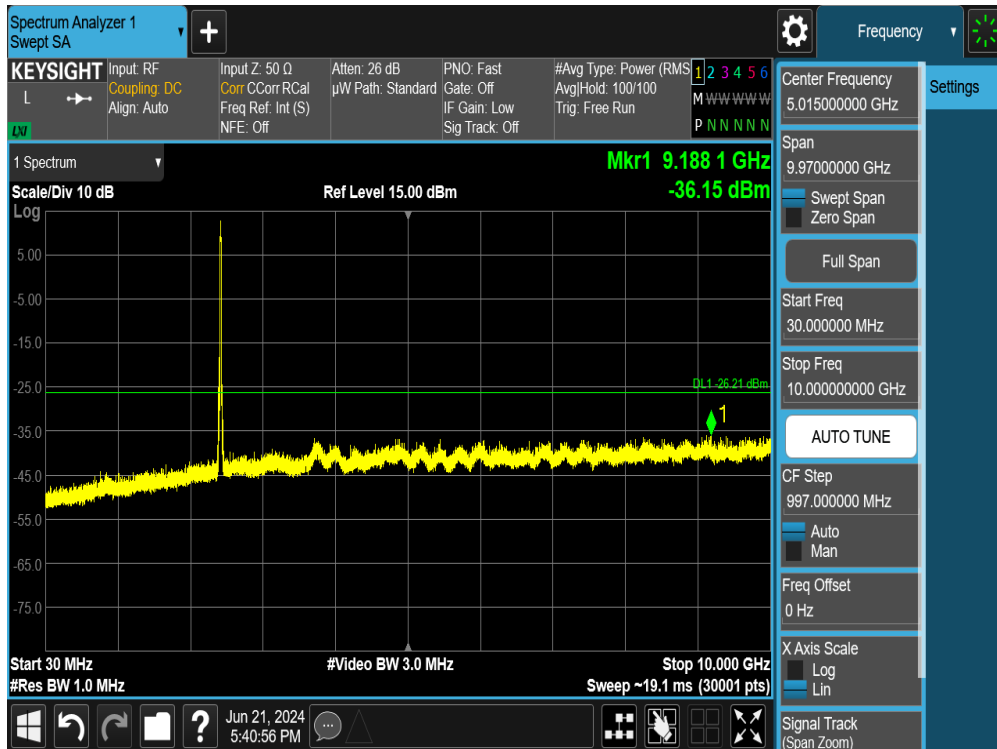
Plot 7-97. Conducted Spurious Plot MIMO ANT1 (802.11ax OFDMA – 242 Tones – Ch. 6)
