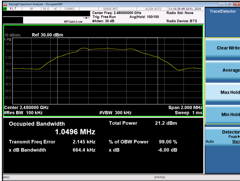
Plot 7-18. 6dB Bandwidth Plot (Bluetooth (LE), 500kbps – Ch. 39 – Ant2)
