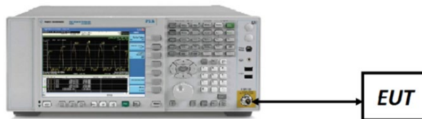
Figure 7-1. Test Instrument & Measurement Setup
