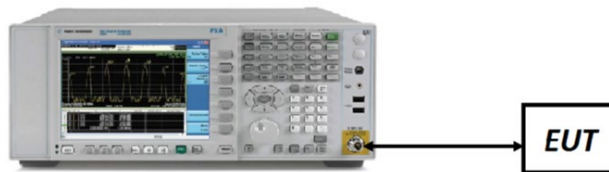
Figure 7-3. Test Instrument & Measurement Setup
