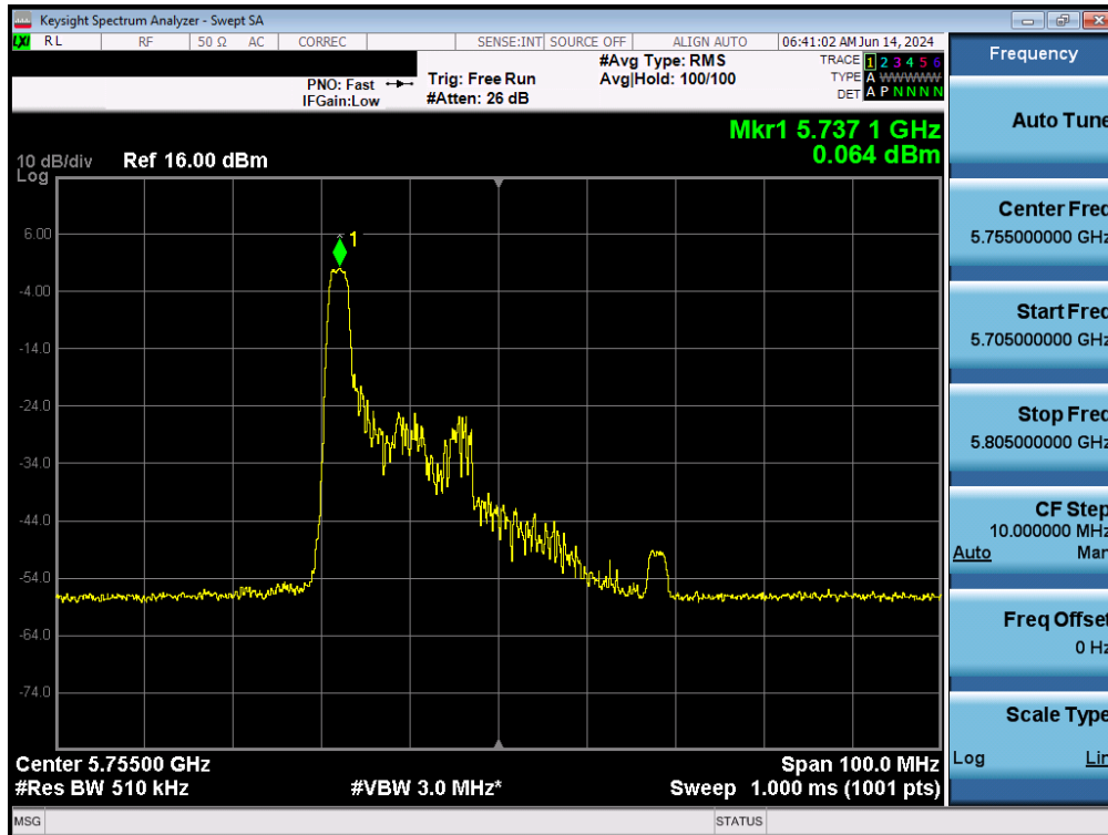
Plot 7-121. Power Spectral Density Plot MIMO ANT2 (40MHz BW 802.11ax – 26 Tones (UNII Band 3) – Ch. 151)
