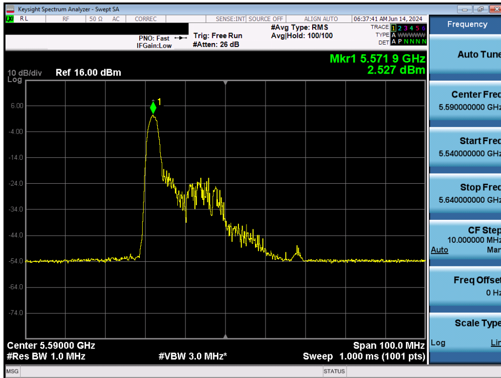
Plot 7-117. Power Spectral Density Plot MIMO ANT2 (40MHz BW 802.11ax – 26 Tones (UNII Band 2C) – Ch. 118)
