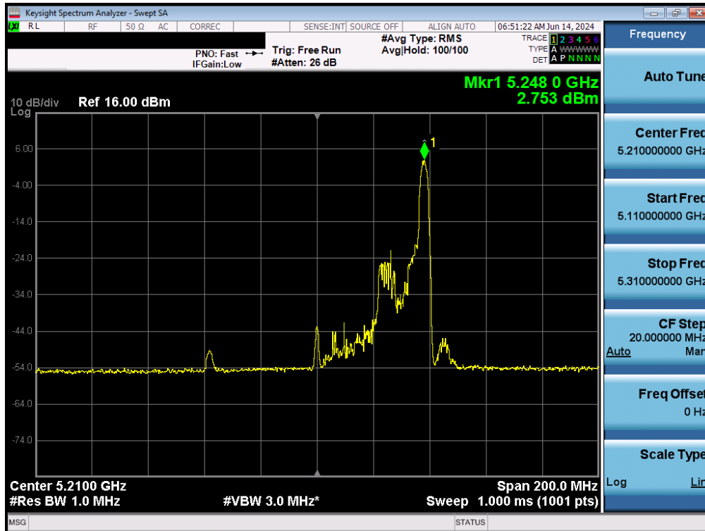
Plot 7-111. Power Spectral Density Plot MIMO ANT2 (80MHz BW 802.11ax – 26 Tones (UNII Band 1) – Ch. 42)
