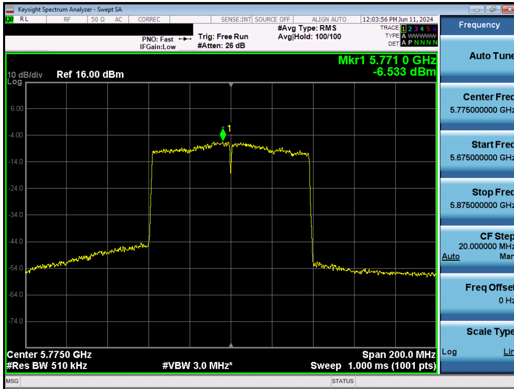
Plot 7-154. Power Spectral Density Plot MIMO ANT2 (80MHz BW 802.11ac (UNII Band 3) – Ch. 155)
