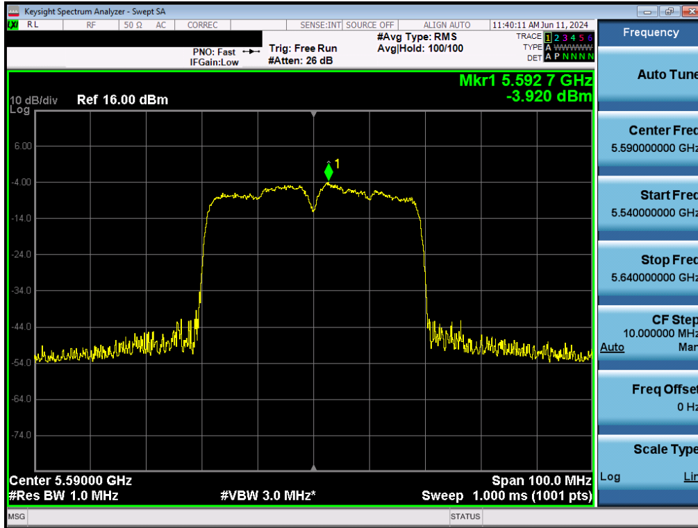
Plot 7-144. Power Spectral Density Plot MIMO ANT2 (40MHz BW 802.11ax (UNII Band 2C) – Ch. 118)
