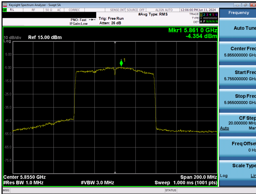
Plot 7-161. Power Spectral Density Plot MIMO ANT2 (80MHz BW 802.11ac (UNII Band 3/4) – Ch. 171)
