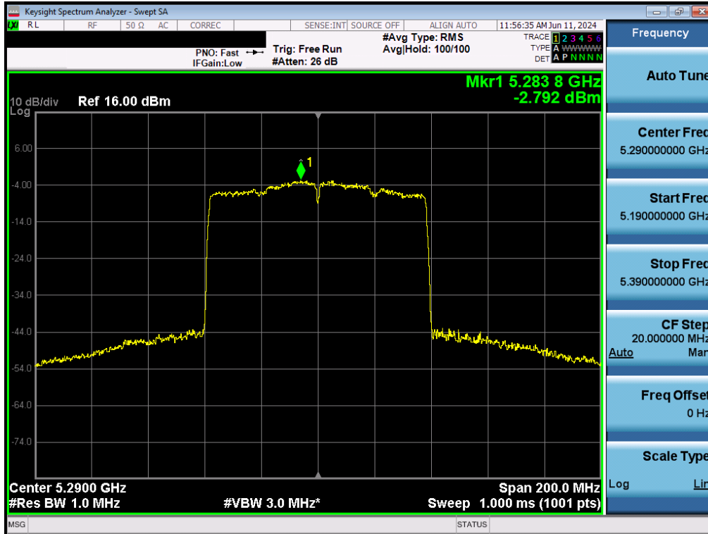
Plot 7-138. Power Spectral Density Plot MIMO ANT2 (80MHz BW 802.11ac (UNII Band 2A) – Ch. 58)
