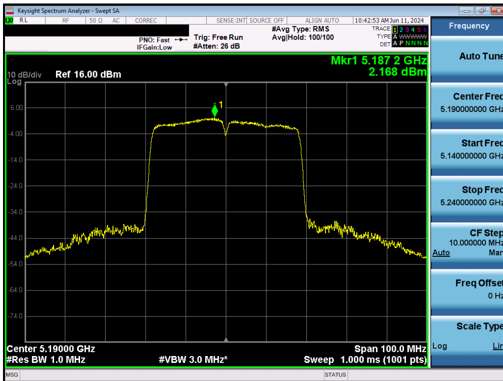
Plot 7-127. Power Spectral Density Plot MIMO ANT2 (40MHz BW 802.11n (UNII Band 1) – Ch. 38)
