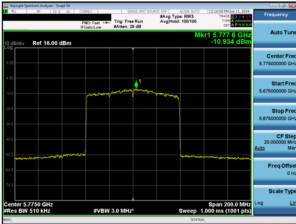
Plot 7-155. Power Spectral Density Plot MIMO ANT2 (80MHz BW 802.11ax (UNII Band 3) – Ch. 155)
